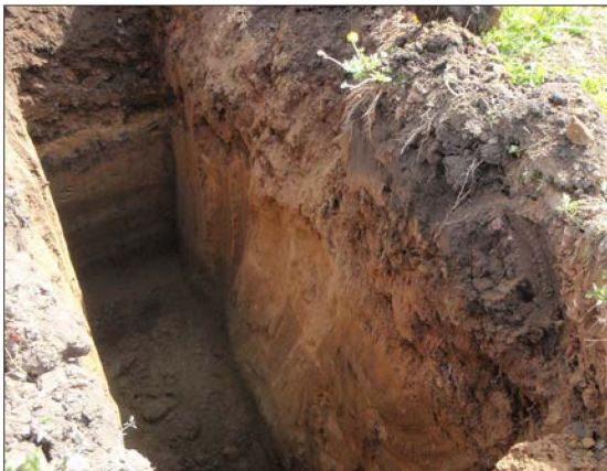
Plate 3: TP22 3.1 m deep, note sand make-up layer 005.
