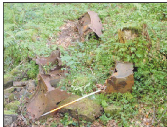
Plate 10: Remnants of the water wheel metal paddles which would have driven the earlier turbine.
