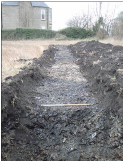
Plate 7: Coal and shale debris visible in trenches 6, 7, 12 and 13 at the west side of the north field, from the east.
