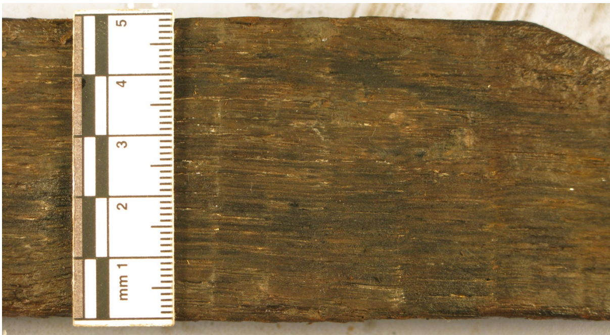
Figure 59 Photograph of saw marks on timber 69
