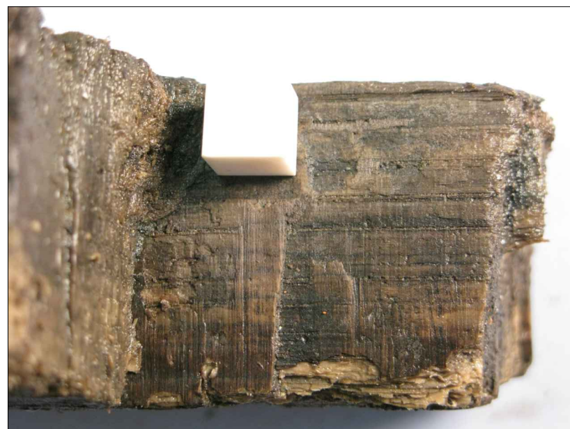
DP34 - Timber 3, Saw Marks - Hi Res Photo
