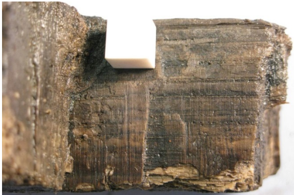
Figure 14 Photograph of saw marks on timber 3. Scale=1cm
