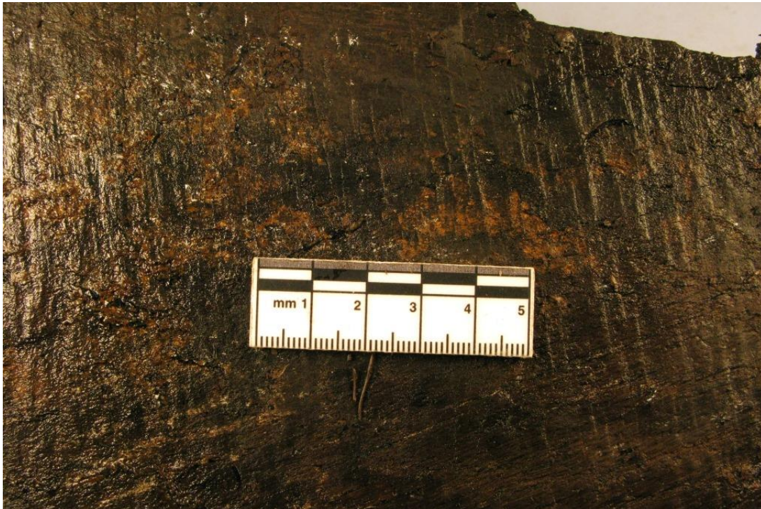
Figure 51 Photograph of saw marks on timber 66
