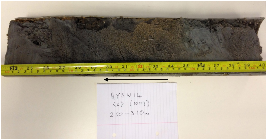
Figure 1 – Photograph of the basal core segment from ABH5 at Sadds Wharf, Maldon (HYSW14) <2> showing the stratigraphy and location of the pollen sub-samples at 2.65m and 2.95m. The arrow points to the top of the core.
