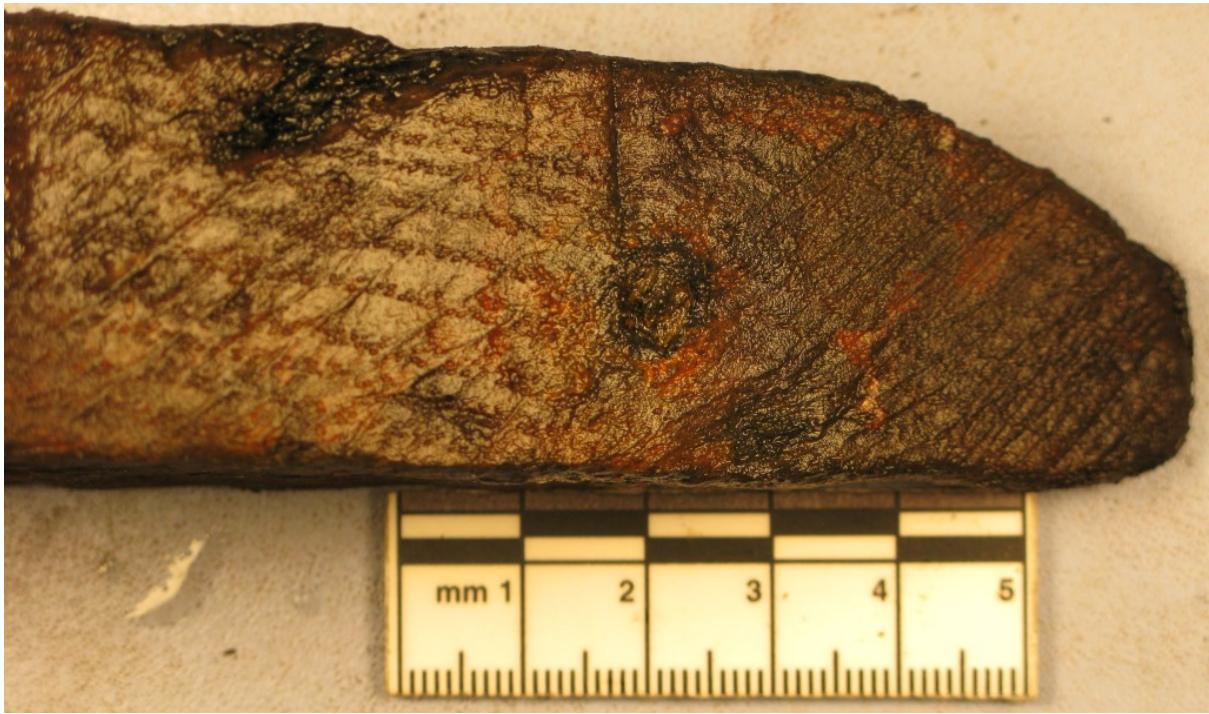
Figure 62 Photograph showing growth rings, iron fitting and saw marks on timber 69
