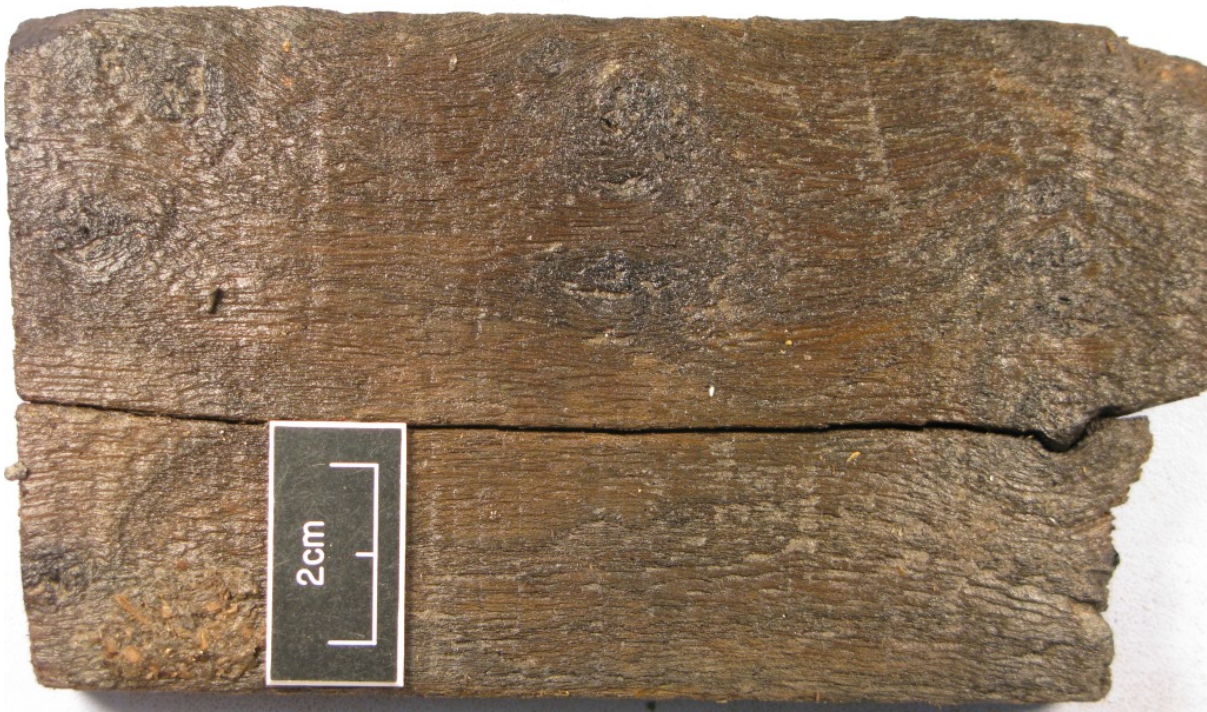
Figure 55 Photograph of saw marks on timber 67
