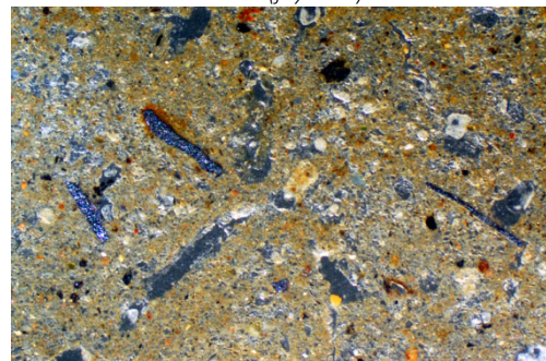
Image 7. As Image 6, under OIL; iron splinters can be interpreted as hammerscale from iron working, as found around industrial hearths elsewhere.
