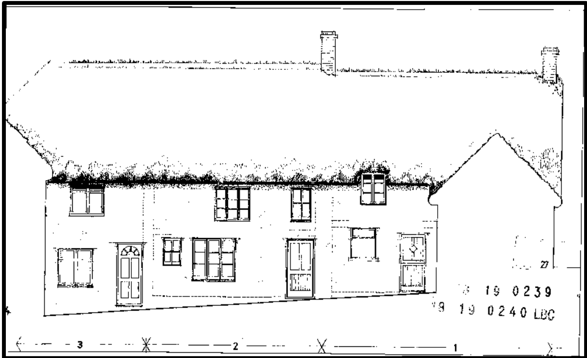
Fig. 4 Reconstruction of the courtyard (north-west facing) elevation of the houses made following the fire in 2012 by Edward Holden, Architect, and submitted as 'as existing' drawings with the current application. Note the change in the ridge line between No. 1 and Nos 2-3.
