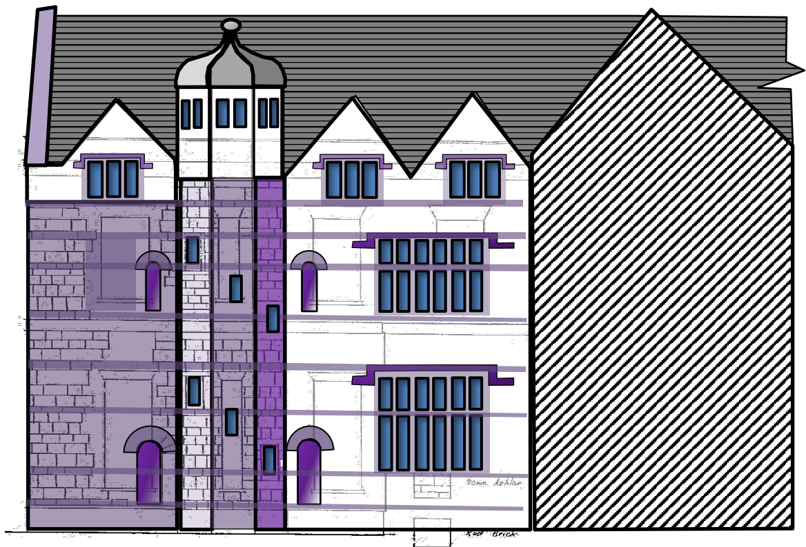
Fig. 15 Possible interpretation of the above drawing, showing a reconstruction of the east face of the western wing of the Elizabethan house, based on 16th- and 17th-century houses elsewhere (including the stair turret and gabled roofline at Poltimore House) with narrow courses emphasised as evidence for string courses, transoms, sills and drip moulds.
