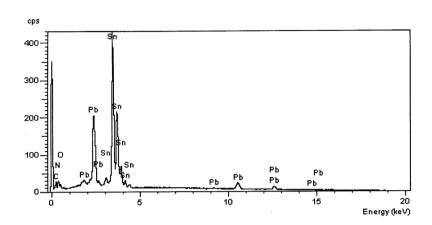
For each of the three samples a semi-quantitative analysis was carried out to determine the approximate ratio of the Pb and Sn used in the alloy. Calibration was carried out against a cobalt standard and area readings taken at 1000x magnification at 2 different areas of the sample surface.
