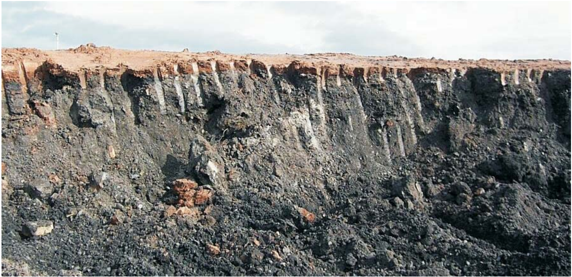
Plate 3 - detail of the section through the redeposited colliery wastes on area 2 (note no sign of ground surface at bottom of profile)
