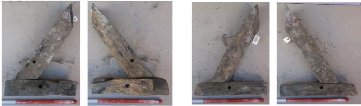
Plates 28-29 Rafter-foot assemblies 001 and 002
