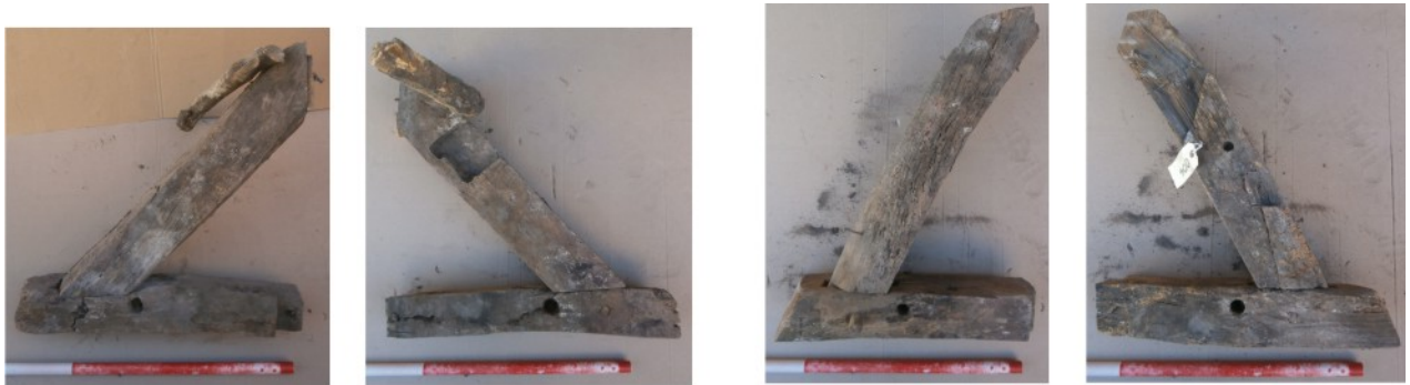
Plates 30-31 Rafter-foot assemblies 003 and 004
