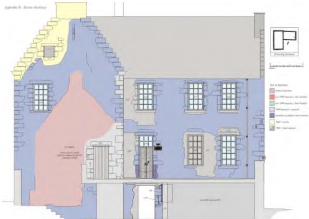
Figure 9 Phased south elevation
