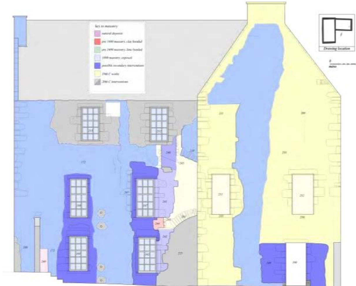
Figure 7 phased north exterior elevation
