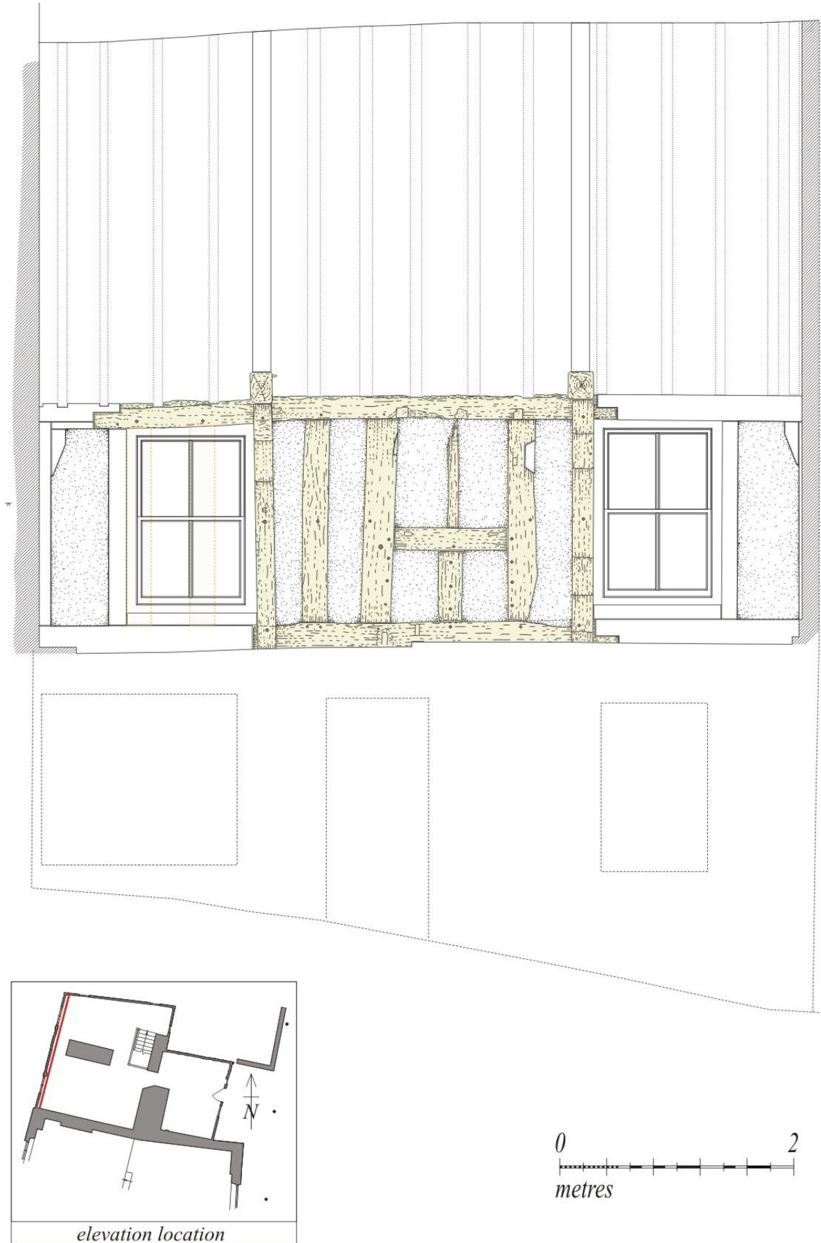
Figure 5 First floor – record of the interior of the west wall
