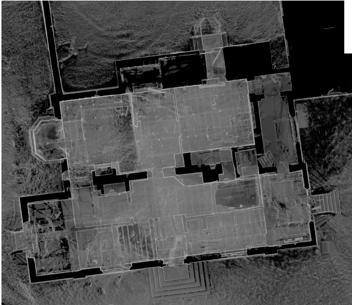
Figure 4 Merged scan imagery – basement and ground floor levels overlain
