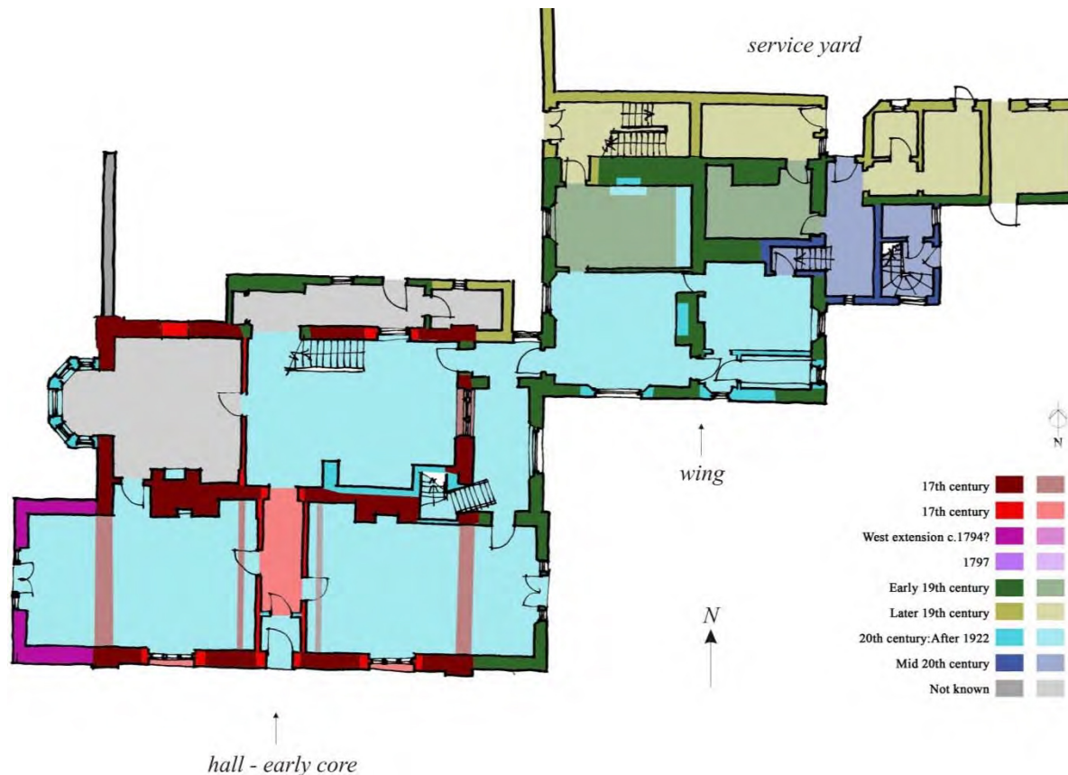
Figure 3 Phase plan at ground floor level – a preliminary interpretation from the 2013 Conservation Plan, with amendment
