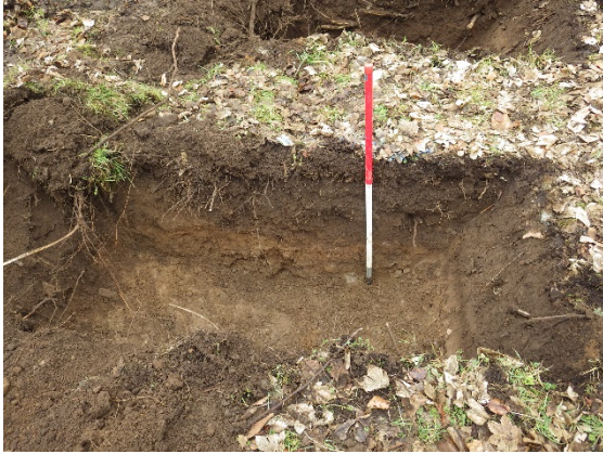
Plate 1 Percolation Pit 1, north facing section showing the structure found in all the pits
