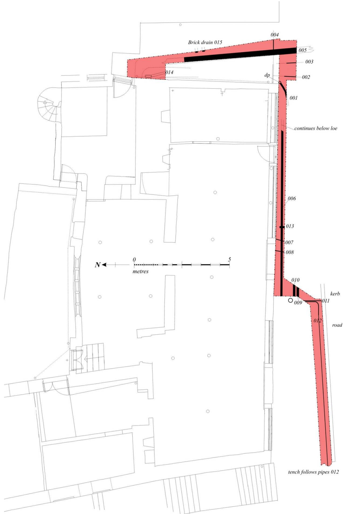
Figure 13 Exterior service trench location plan
