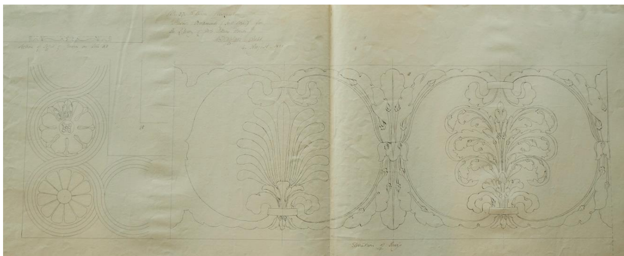
Figure 20 William Playfair ground floor Room G.2 (Library) cornice and frieze detailings. University of Edinburgh CRC, Coll-13/10, no. 941
