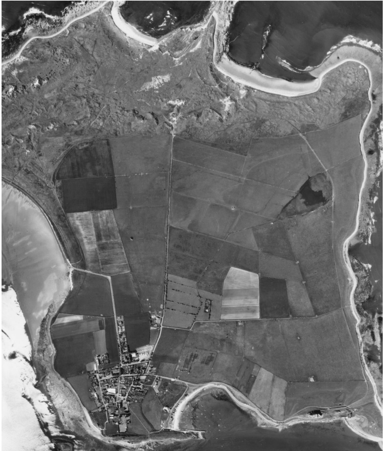
Figure 13: 1977 vertical aerial photograph, showing the full extent of the tramway leading from the quarry at Nessend to the kilns at Castle Point.
