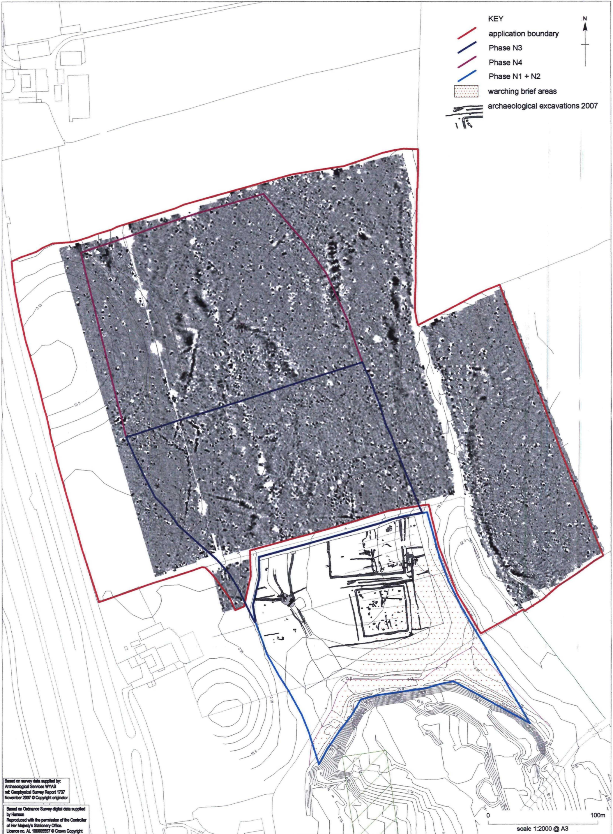
Figure 2 Allerton Park Quarry: greyscale magnetometer data and topographic detail
