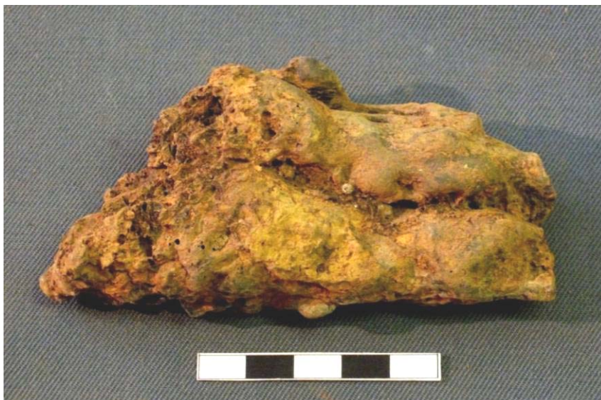
Tap slag from the tapping holes of a smelting furnace (Scale 50mm) Fig 46
