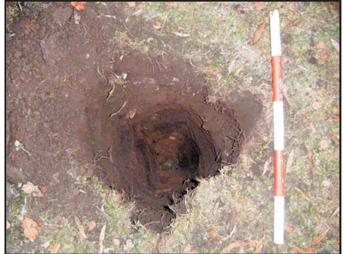
Illus 22: The hand-dug hole at a depth of 1.2m before the commencement of boring.
