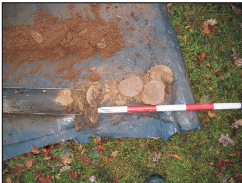
Illus. 20: Sandstone present at a depth of c.1 metre in Borehole 5.
