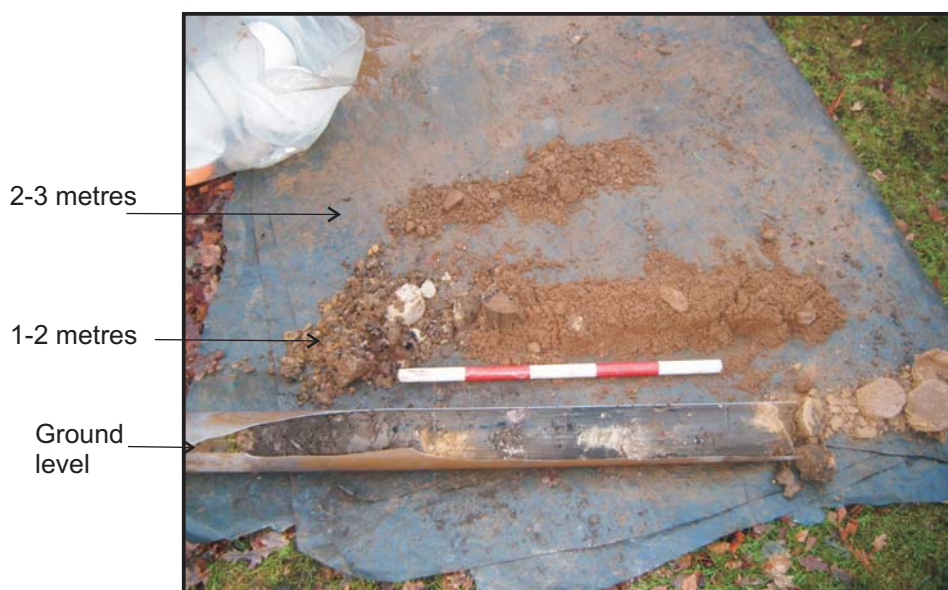
Illus. 19: The core produced from Borehole 5.
