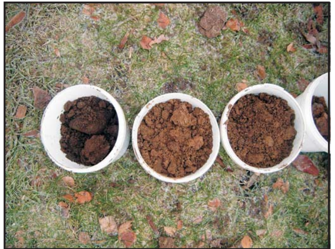
Illus 24: Samples from Borehole 6 taken from c.1.5 - 3m below ground level.
