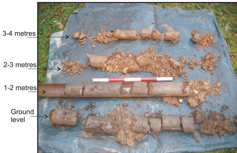
Illus. 08: The core produced from Borehole 1.
