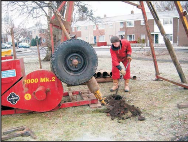
Illus 21: The hand-dug first phase of Borehole 6, viewed from the north-east.
