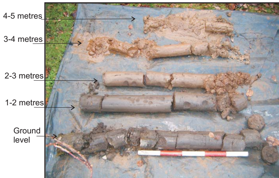
Illus. 11: The core produced from Borehole 2.
