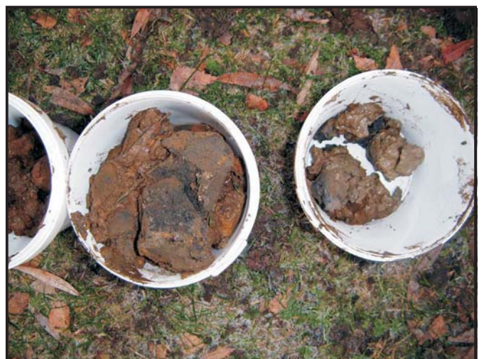
Illus 26: Samples taken from c.5 - 6m below ground level, showing clay-based deposits.
