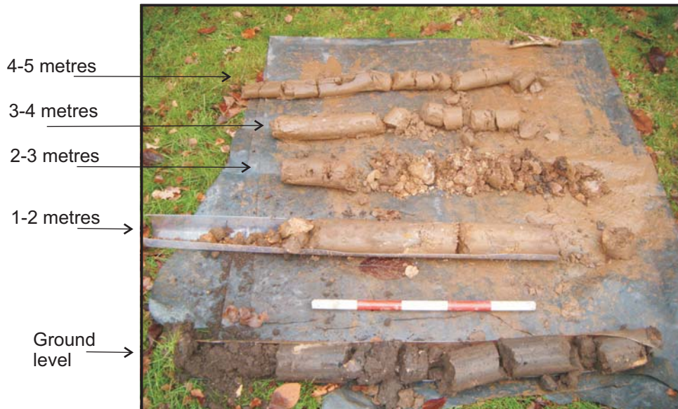
Illus. 14: The core produced from Borehole 3.
