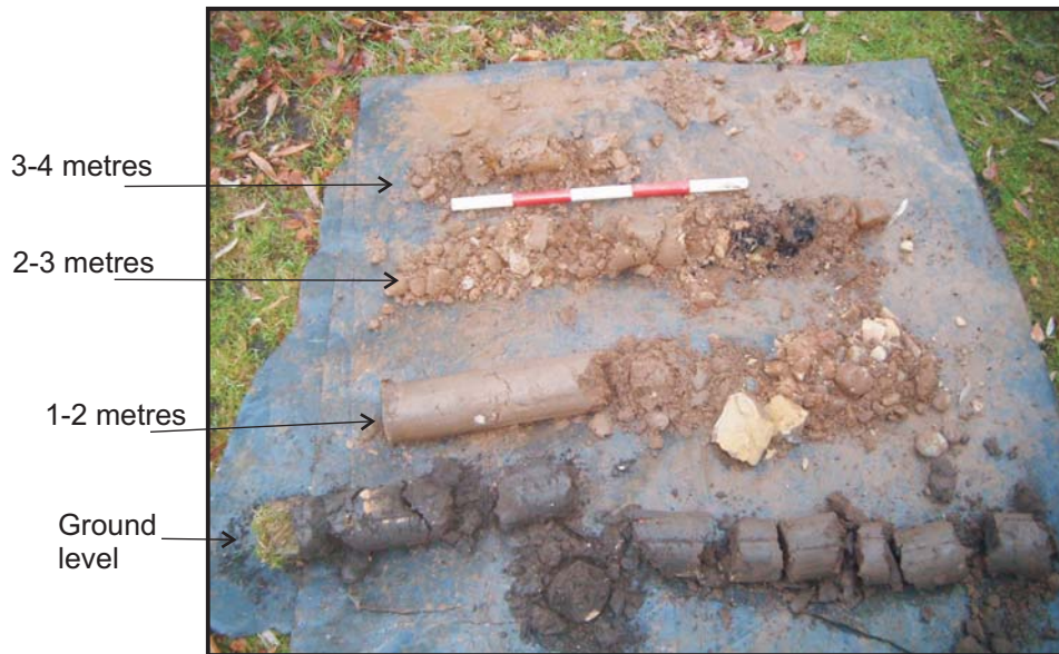
Illus. 16: The core produced from Borehole 4.
