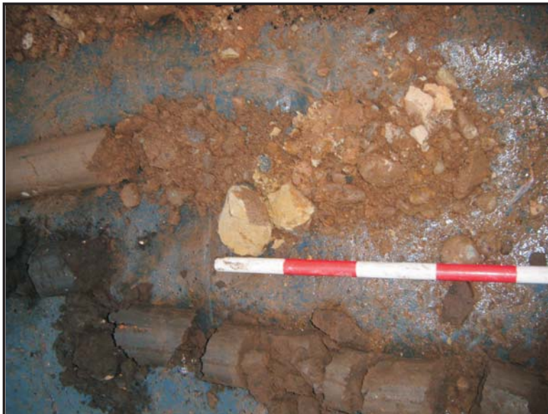
Illus. 17: Sandstone present at c.1.5metres in Borehole 4.
