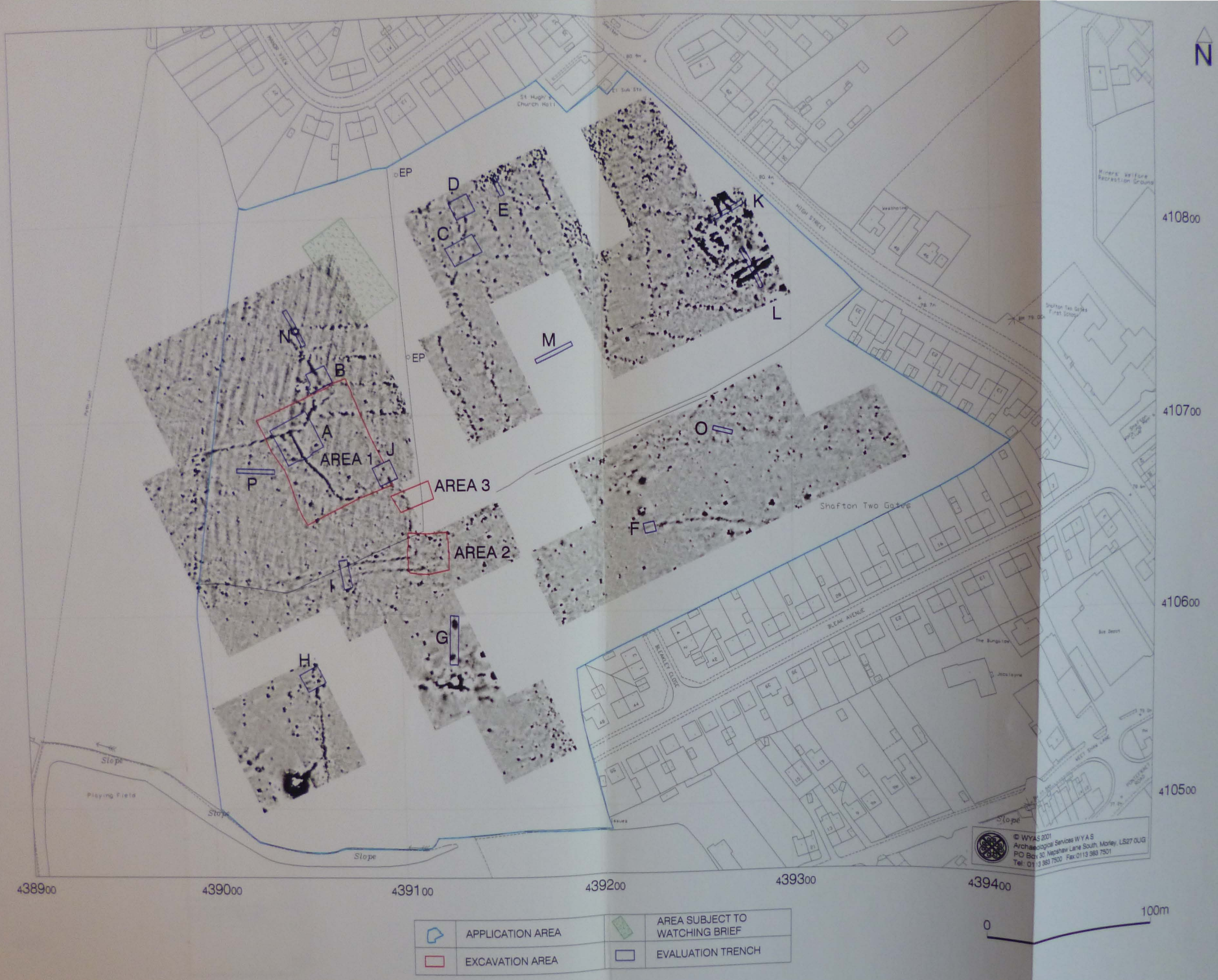
Fig. 2. Site location showing gradiometer greyscale data and trench locations
