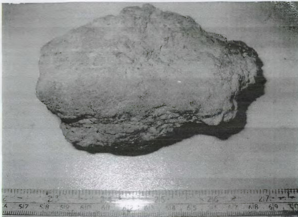
Figure 1.2 More typical example of a Fulford Hearth Bottom but still lacking the upper surface concave shape most commonly found in samples of this type
