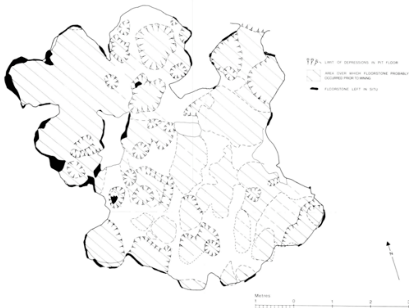
Figure 14 1971 Shaft pit floor. Configuration and location of extracted floor stone nodules
