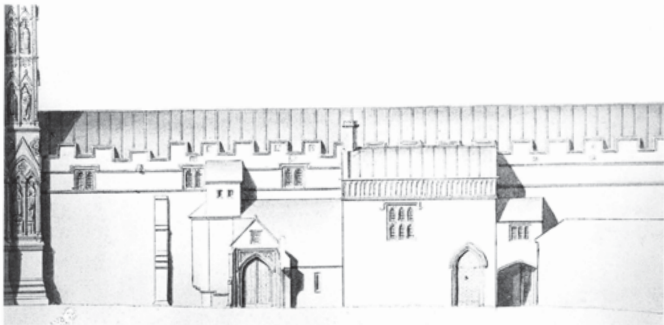
Fig. 341 Garter's elevation of the west cloister, c. 1795, showing the two porches but omitting later additions (Courtesy of the Society of Antiquaries of London)
