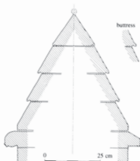
Fig. 290 Section through the early thirteenth-century coping and string-course of the south cloister wall. The inset shows the kicked weathering-groove found on the copings of the south cloister buttresses. Scale 1:10
