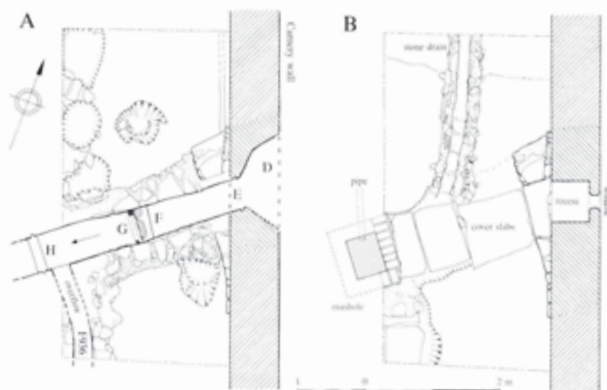
Fig. 398 Plans of excavation Area 8 and the adjoining Camery wall. A Late medieval features. The conduit is shown without its cover-stones. B Post-medieval features. Scale 1:80
