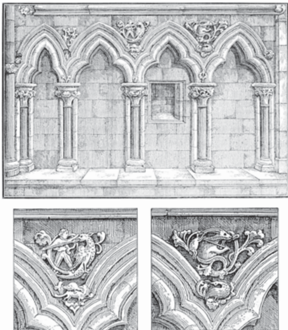
Fig. 155 Bristol Cathedral, Elder Lady Chapel. Wall arcading with sculptured spandrels, c. 1220. Enlarged views of beasts also shown. After Lysons 1803
