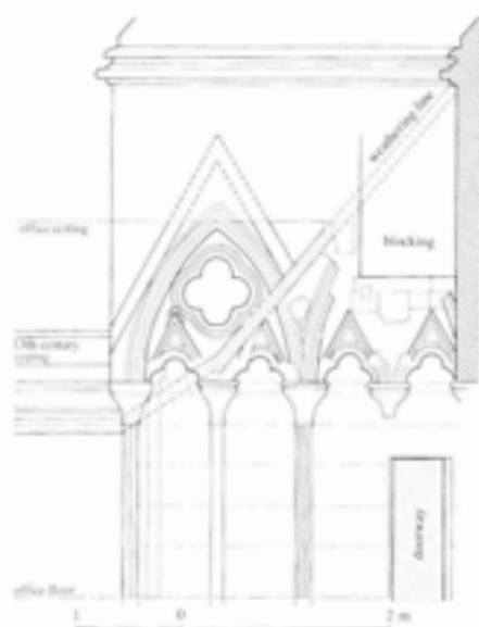
Fig. 286 South-west tower. The east face of the south-west corner buttress, showing the chase of a pentice roof that closed the north end of the west cloister. This is now preserved inside a first-floor office. The thirteenth-century coping to the cloister abutment is shown partly restored; later medieval work is omitted for clarity. Scale 1:80. After Sampson 1998
