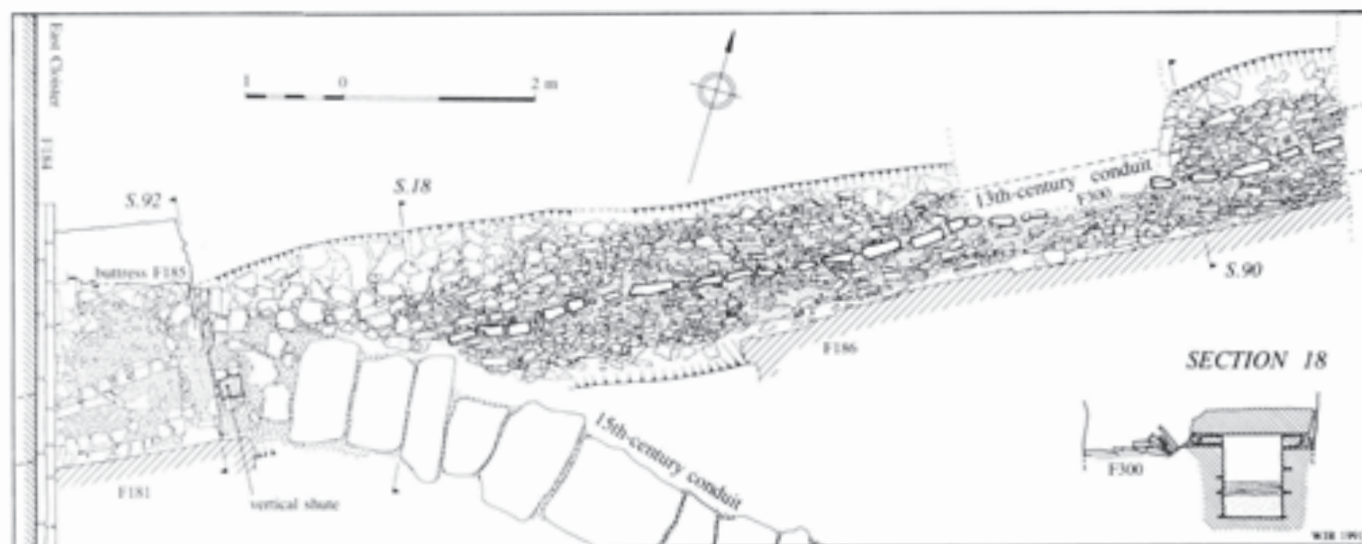
Fig. 391 Plan of the early thirteenth-century conduit (F300) as excavated in Areas 4-5. The junction with Stillington's conduit, entering from the south, is also shown. For sections, see Fig. 392. Scale 1:80
