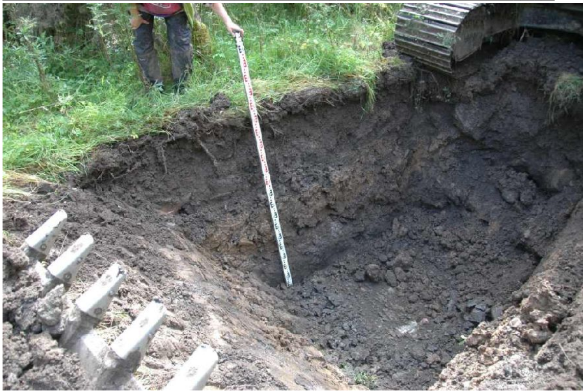
Illus 6 Test pit TP 208 showing redeposited infill material backfilled into borrow pit
