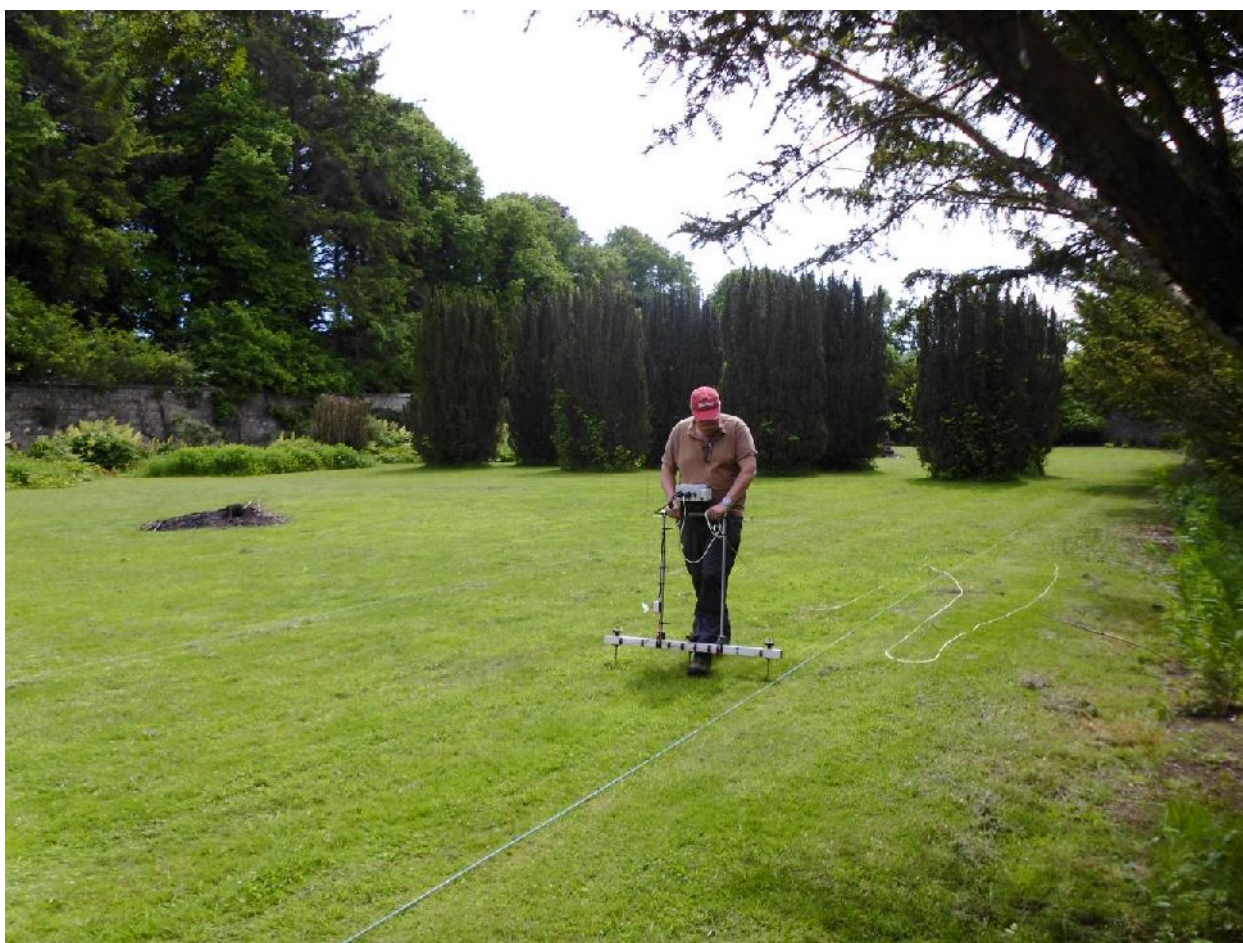
Illus 38 Resistivity survey being undertaken (Photograph courtesy of Rose Geophysical Consultants)
