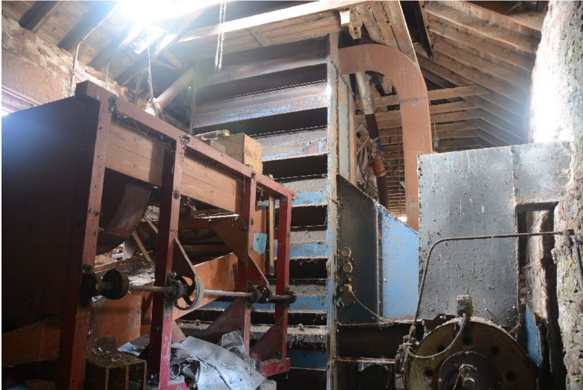
Illus 39 Seed dressing machine (foreground) with grain drier behind.
