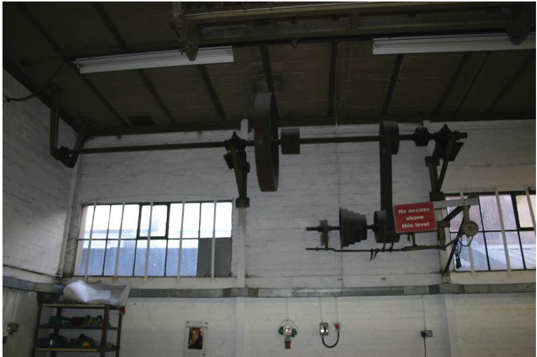
Plate 10: Belt drive power transmission system with gearing in north-east corner
