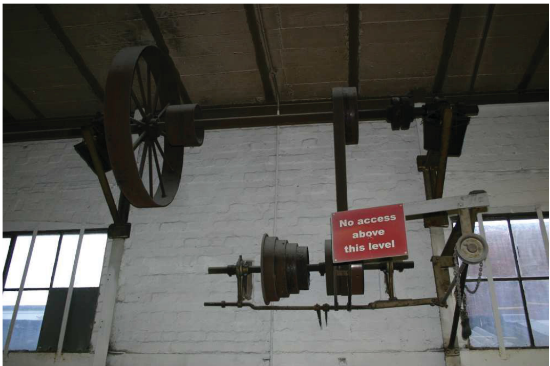
Plate 11: Belt drive power transmission system, detail
