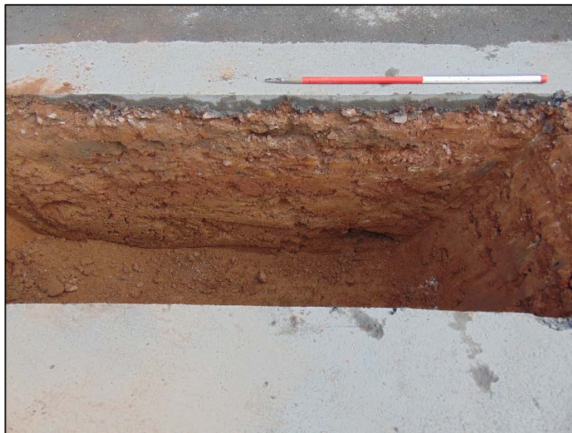
Plate 1; West facing section, Pit D showing made ground deposits, 1m scale.
