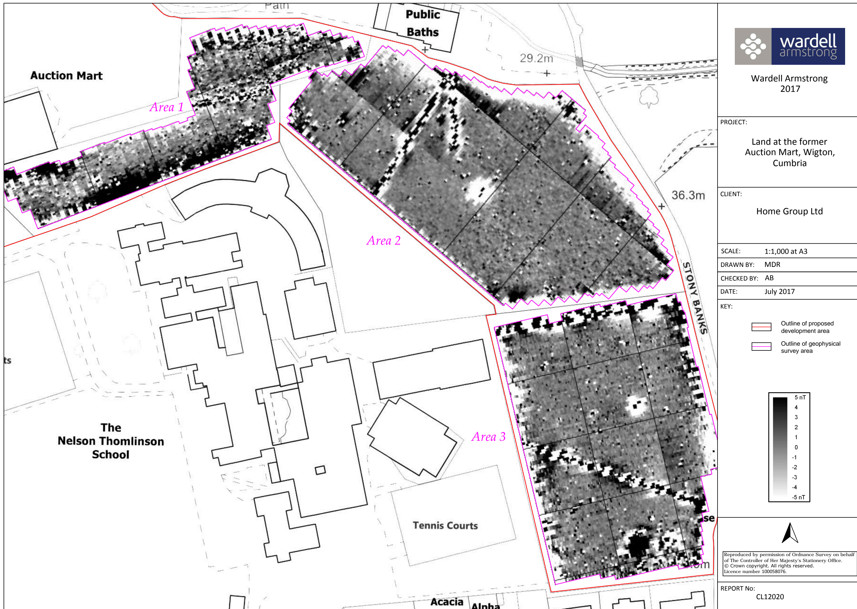
Figure 11: Geophysical survey areas (unprocessed data) showing survey grids.
