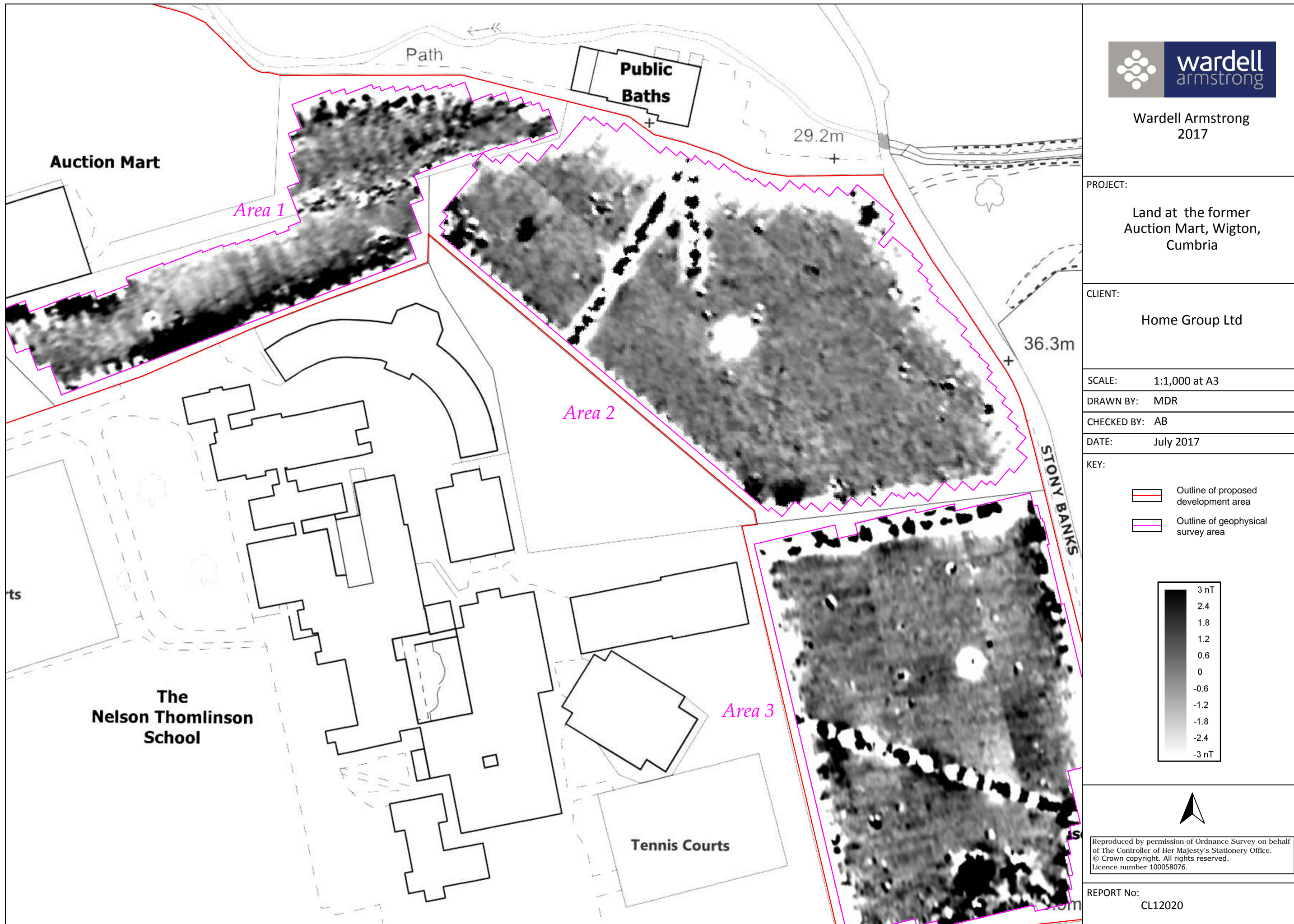
Figure 12: Geophysical survey areas (processed data).
