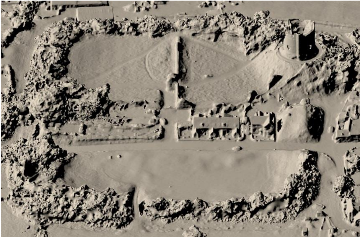
Figure 7: Structure from Motion 3D model of Longtown Castle, (Oblique looking west)
