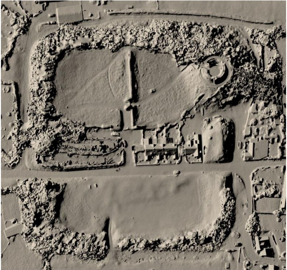
Figure 6: Structure from Motion 3D model of Longtown Castle, (Vertical)
