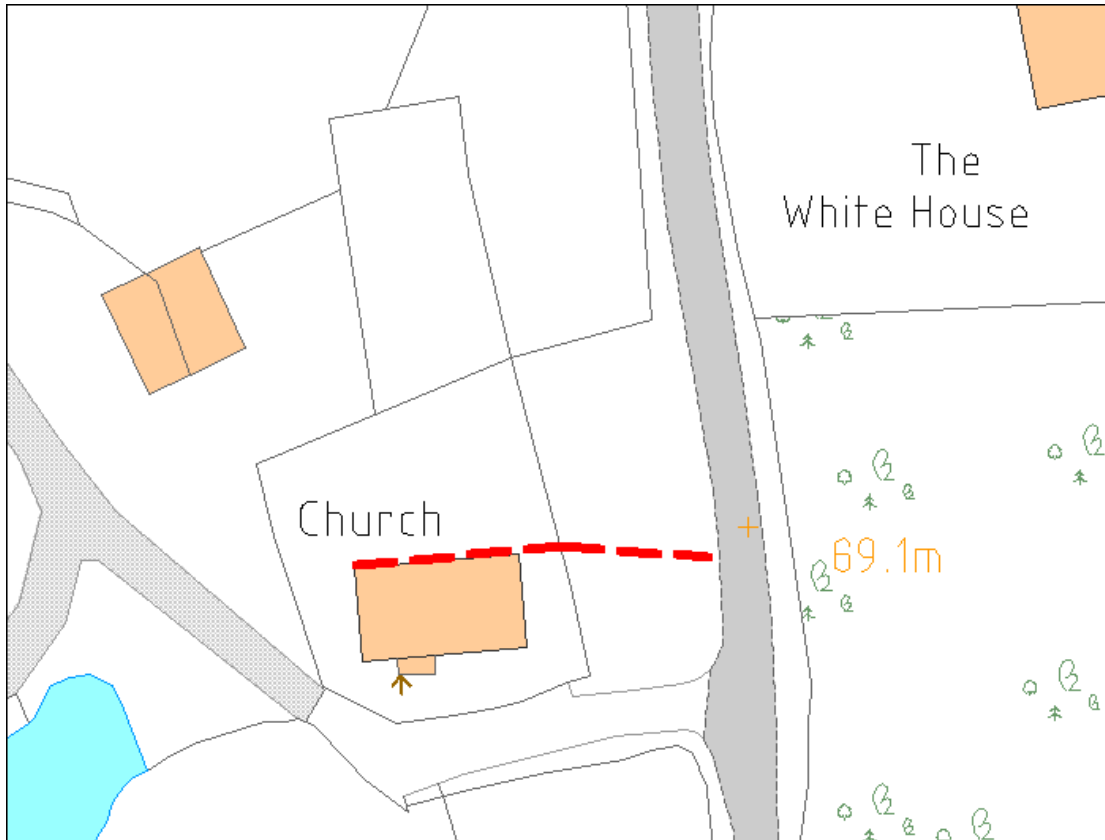
Figure 3: Plan of Aylton Church and churchyard, the drainage run is highlighted as the dashed red line.
