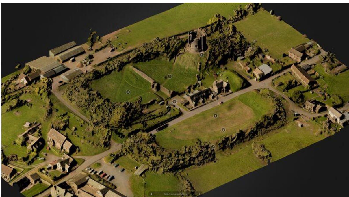
Figure 2: Structure from Motion 3D model of Longtown Castle produced from the drone survey in 2016.
