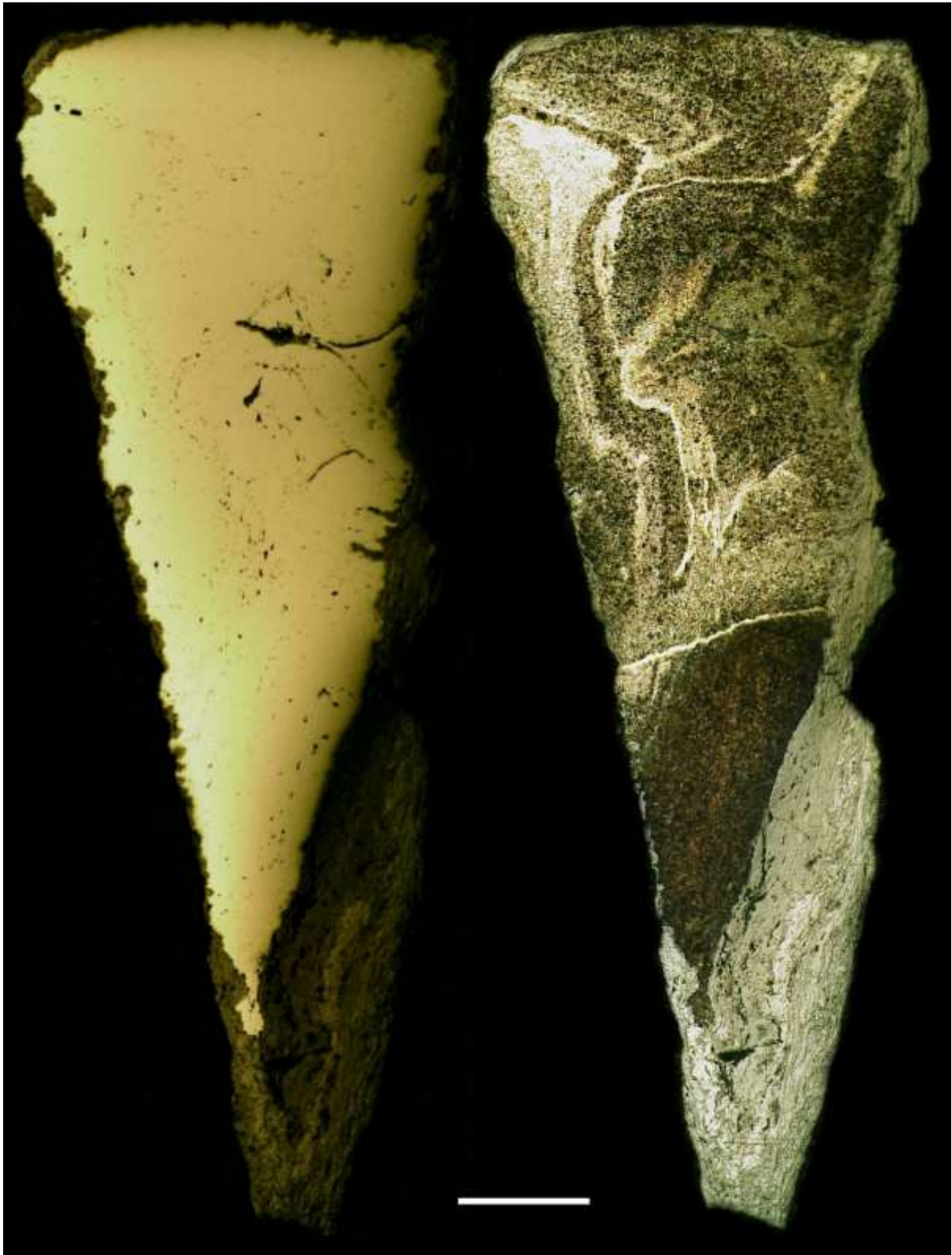
Figure 16: Mapped section of knife 69 in the un-etched (left) and etched condition (right).
