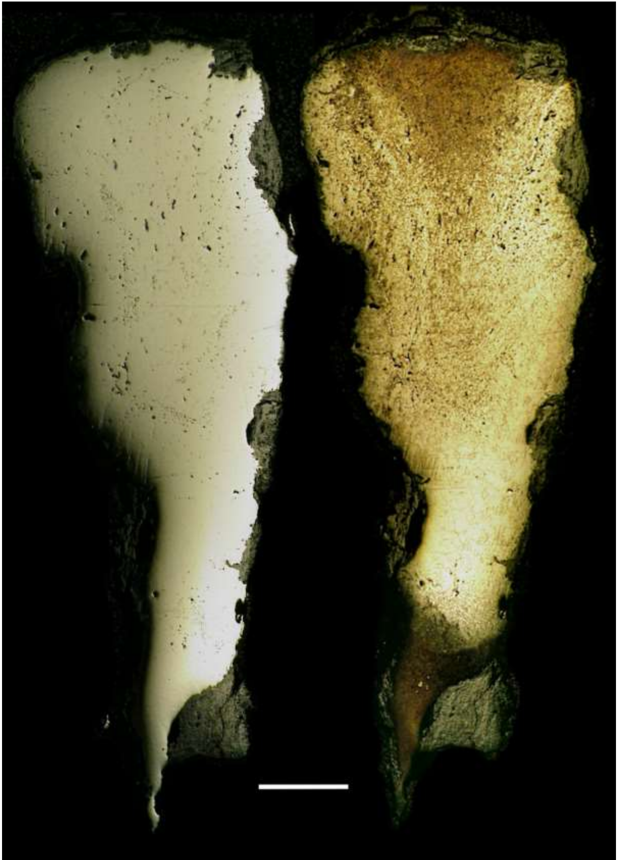
Figure 21: Mapped section near the bent end of knife 75 in the un-etched (left) and etched condition (right).
