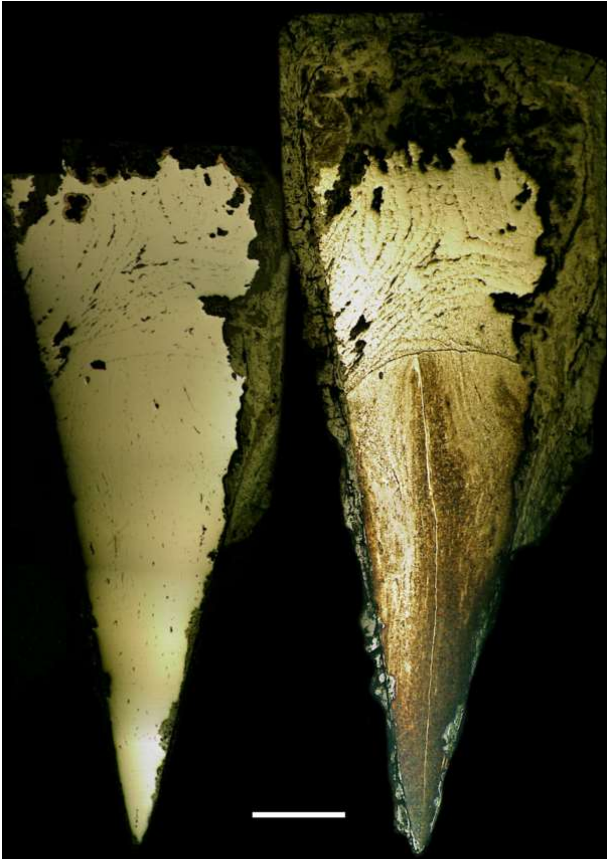
Figure 18: Mapped section of knife 70 in the un-etched (left) and etched condition (right).
