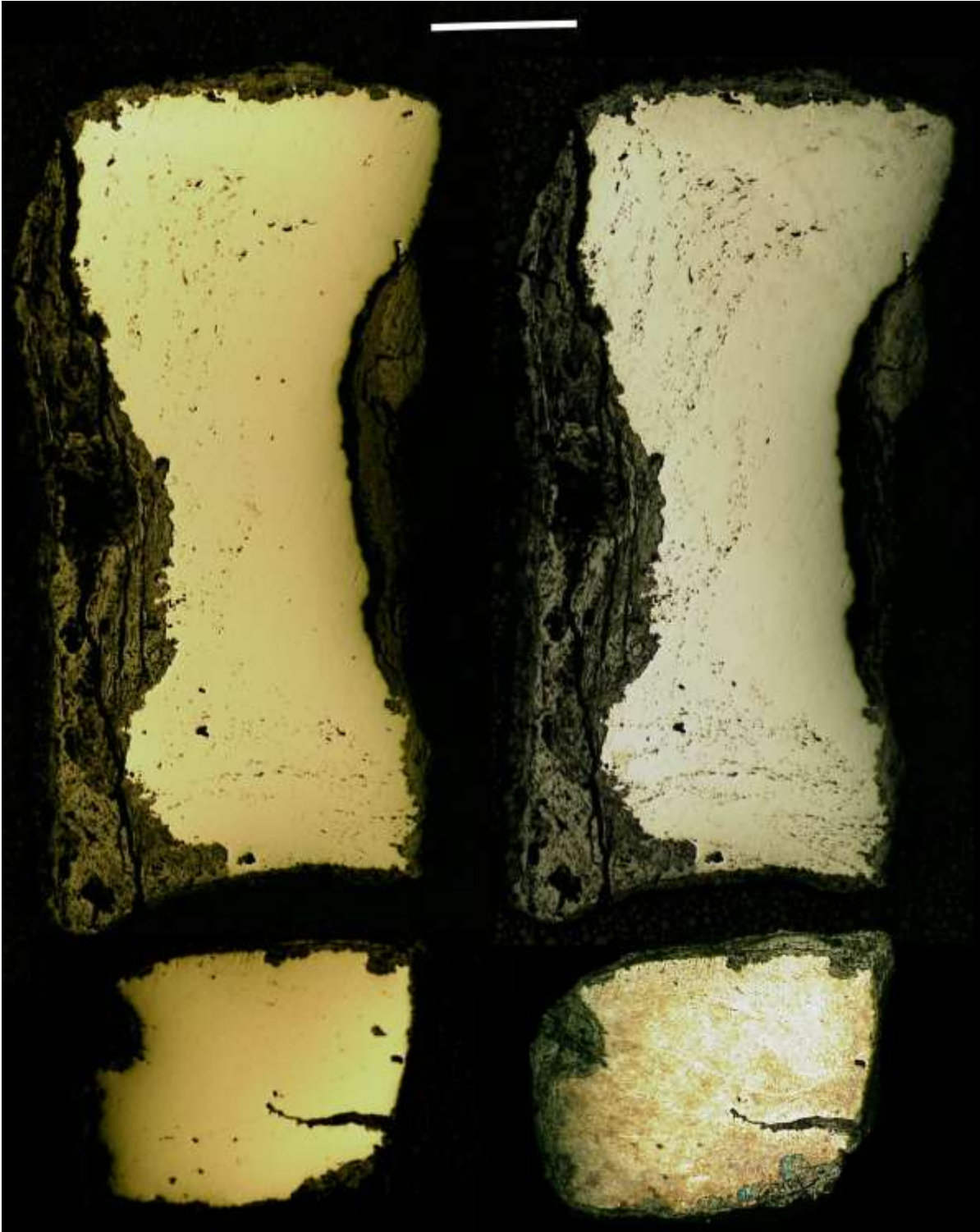
Figure 23: Mapped section of knife 76 in the un-etched (left) and etched condition (right).
