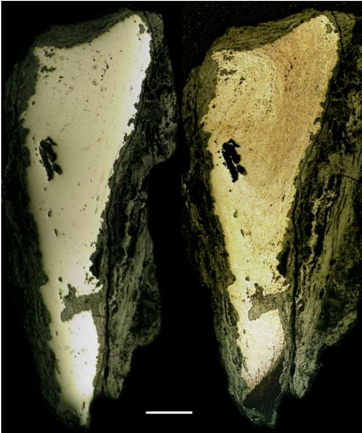
Figure 20: Mapped section of knife 75 in the un-etched (left) and etched condition (right).
