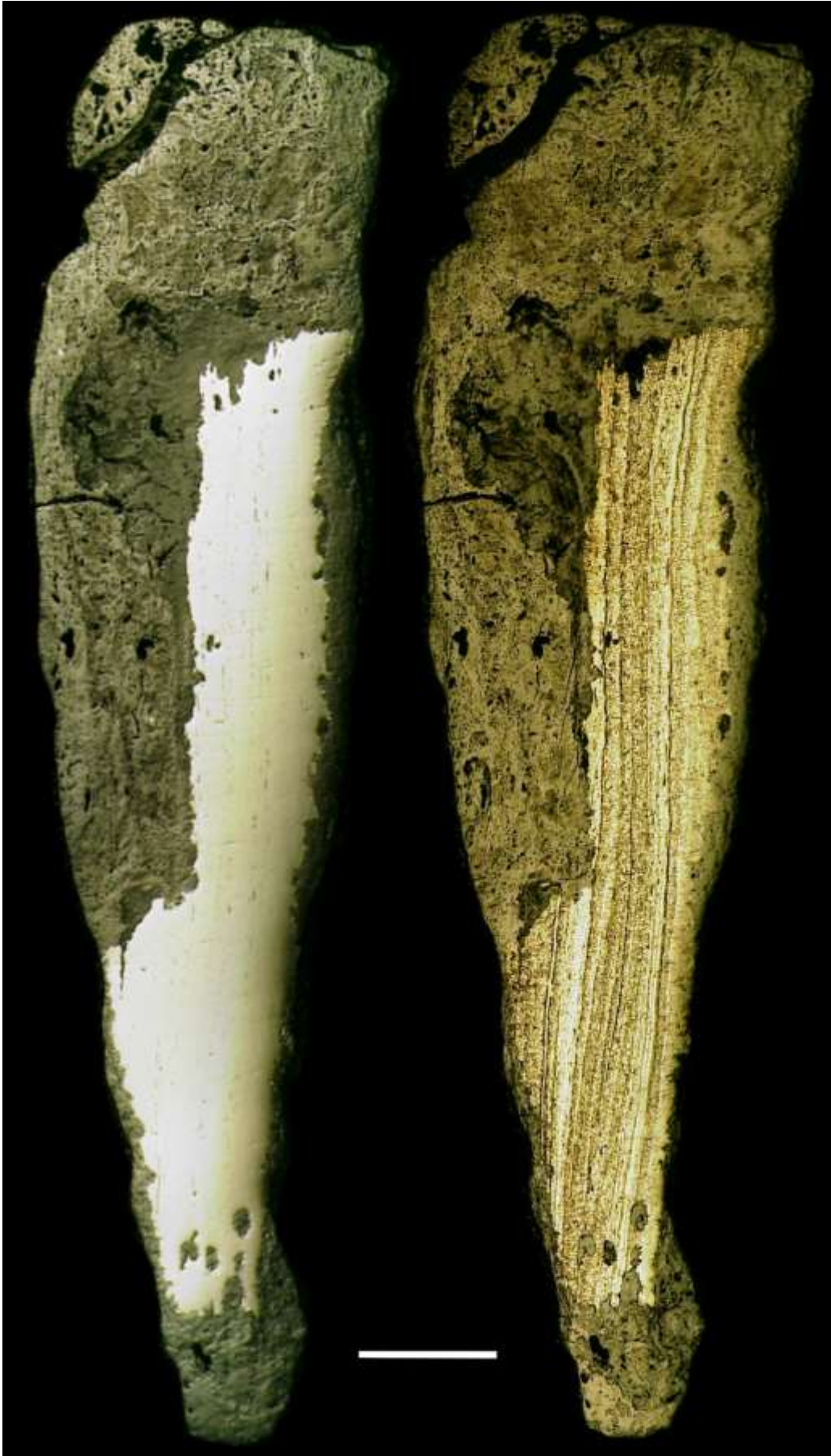
Figure 25: Mapped section of knife 113 in the un-etched (left) and etched condition (right).
