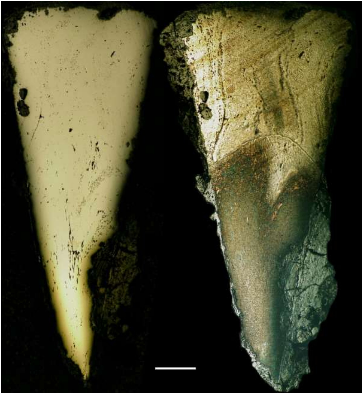
Figure 35: Mapped section of knife 244 in the un-etched (left) and etched condition (right).
