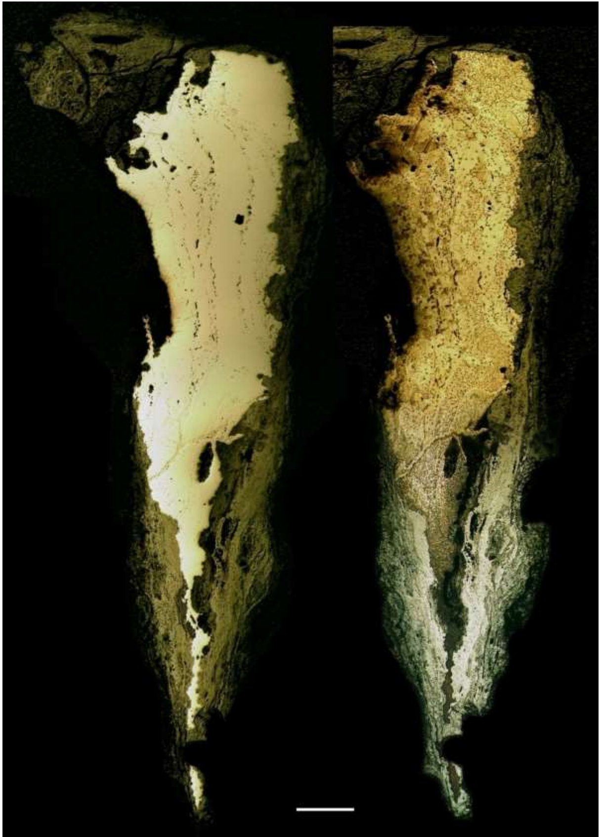
Figure 14: Mapped section of knife 67 in the un-etched (left) and etched condition (right).
