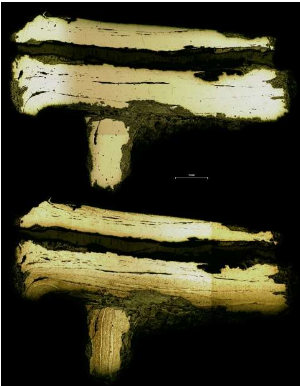
Figure 38: Mapped section of the pivot point in pivoting knife 4 in the un-etched (top) and etched condition (bottom).
