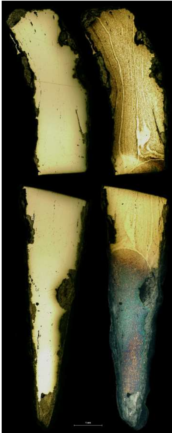
Figure 37: Mapped section of pivoting knife 4 in the un-etched (left) and etched condition (right).
