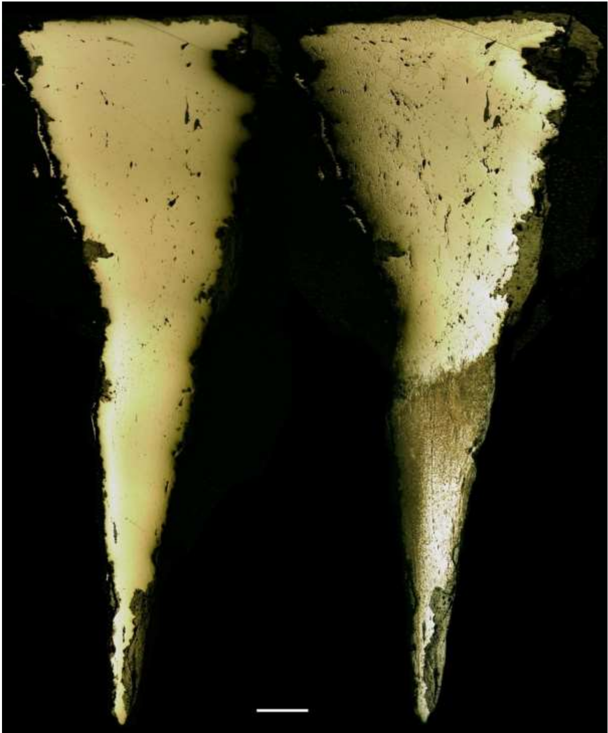
Figure 12: Mapped section of knife 65 in the un-etched (left) and etched condition (right).
