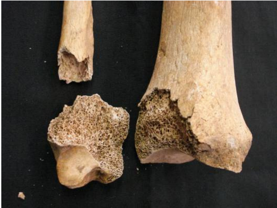
Photo 5. Flaking of tibia of Leg 32 from impact with ankle.
