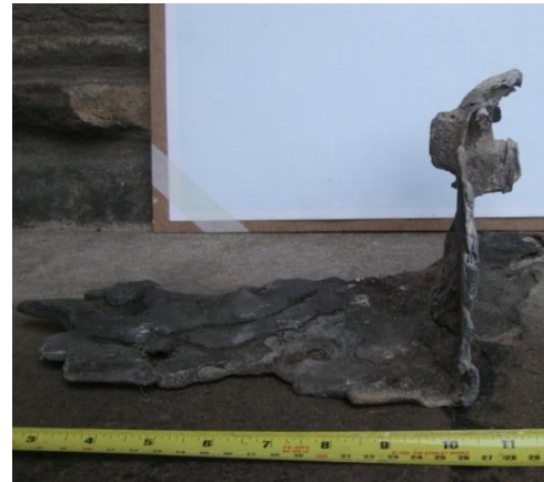
Plate 45 (Archive image PCGC 200) North Portico, top step: the lead cramp extracted. Photograph: Caroline Atkins
