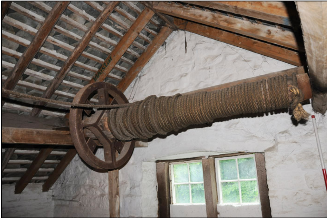
Appendix 3.31: Detail of winch and rope from hoist in ceiling of T1, looking south.
