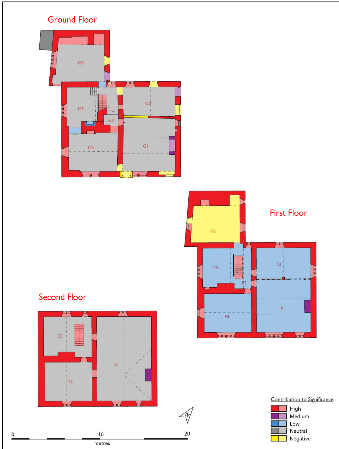
Figure 4: Plan showing the contribution made by fabric to the significance of Woodseats farmhouse.
