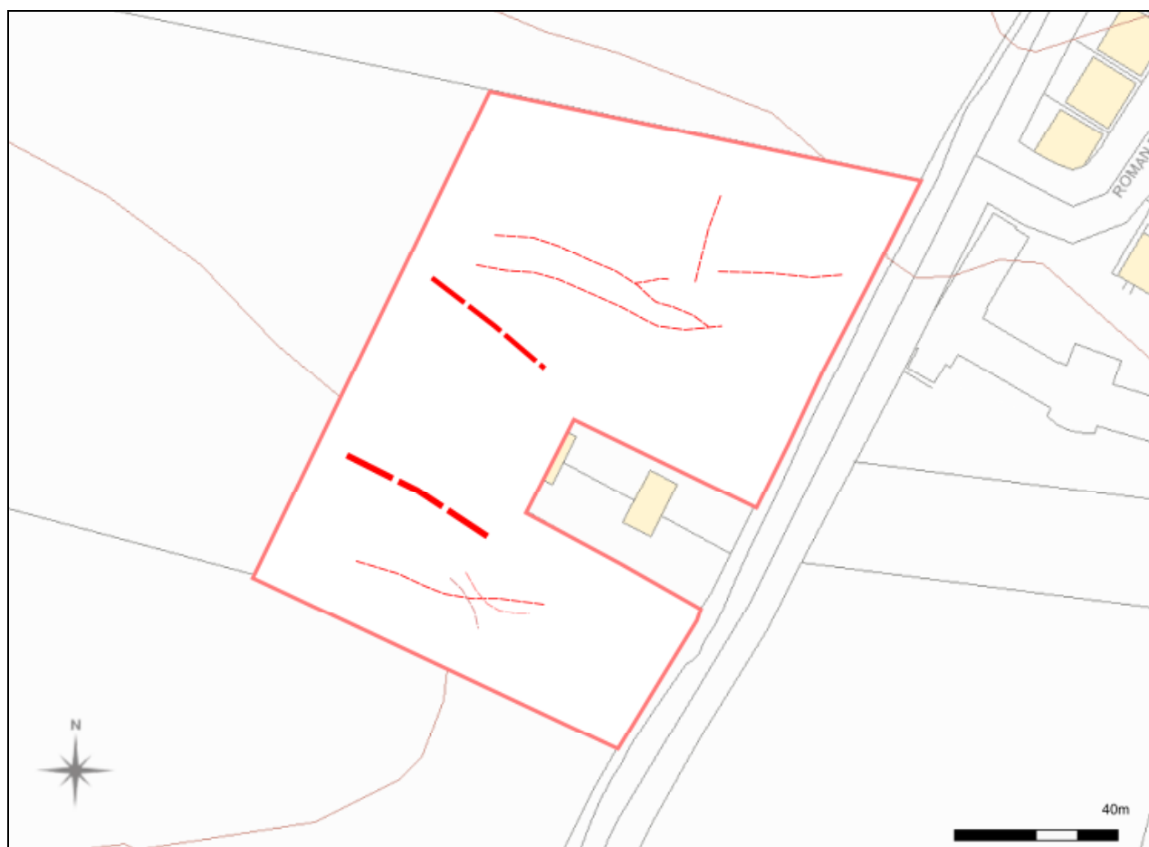
Figure 16. Interpretational plot of possible weak magnetic anomaly responses from the survey
