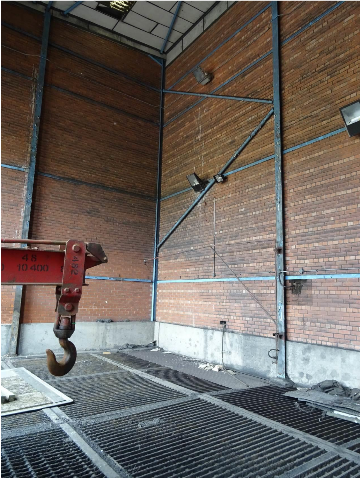
Plate 60. Grading grille which allows coal nuggets to be graded by size
