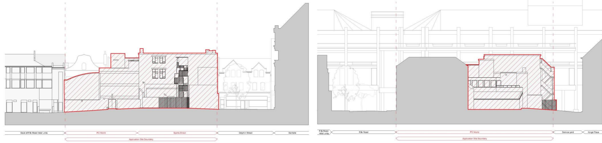
3 Demolition Drawings: Existing South Elevation Scale: 1:200
