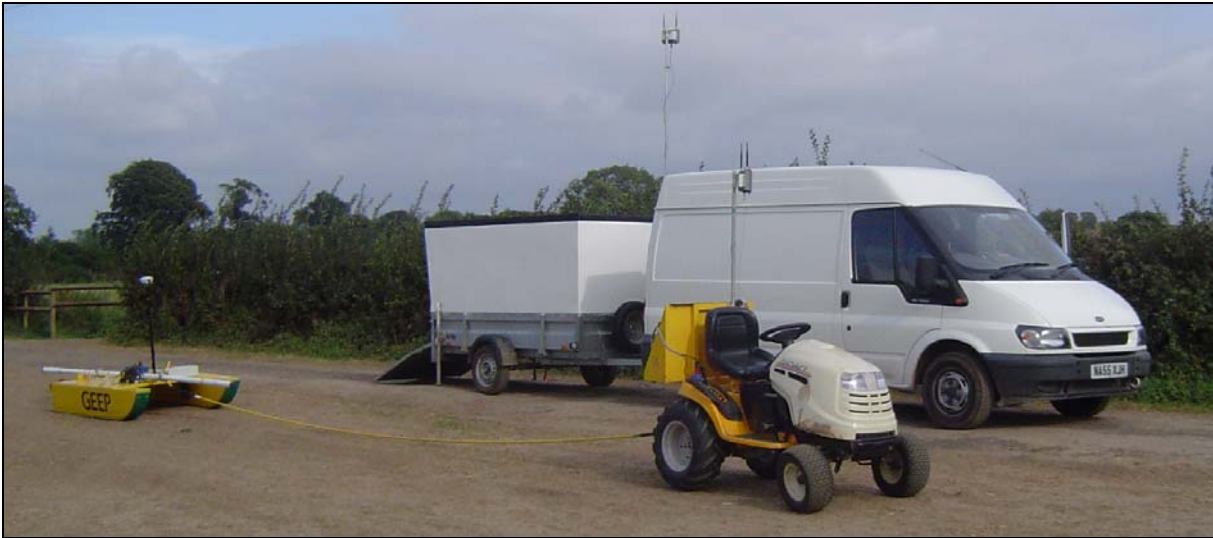
Figure 4.4 The Leicester GEEP system on the Shelford site comprising towing tractor (right), MSP sledge (left, in this case with EM31, and the hired van and trailer (rear) which transports all the equipment and acts as office and workshop on site.
