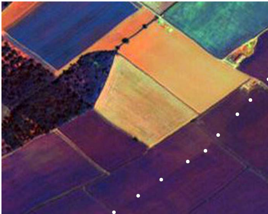
Figure 7.4: False colour composite of NERC ATM image (Bands 11(Red) 10(Green) & (Blue)) showing distinctive signature line of buried "cliff" feature emphasised by white spots over a distance of approximately 600m SW to NE.
