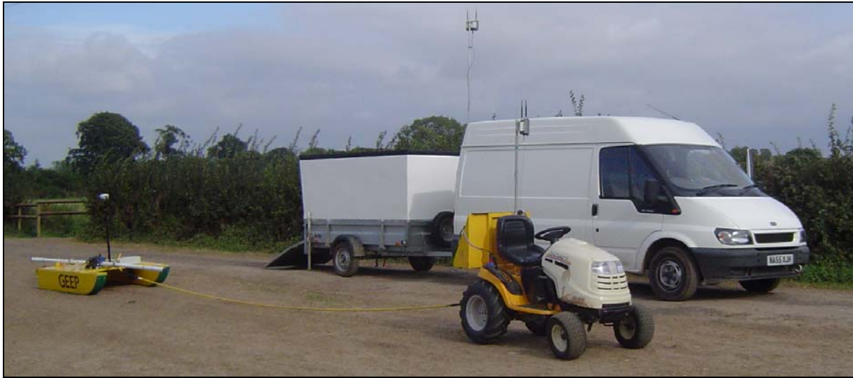
Figure 3.4 The Leicester GEEP system on the Shelford site comprising towing tractor (right), MSP sledge (left, in this case with EM31, and the hired van and trailer(rear) which transports all the equipment and acts as office and workshop on site.
