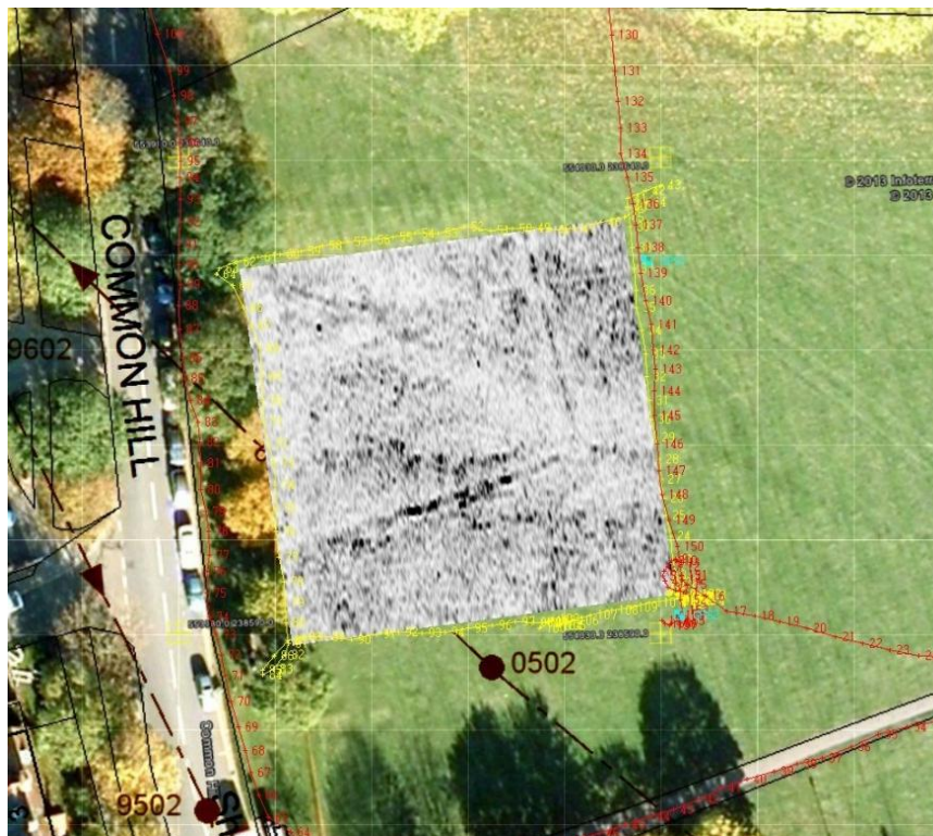
Figure 4: Results of ground penetrating radar survey conducted in 2013.
