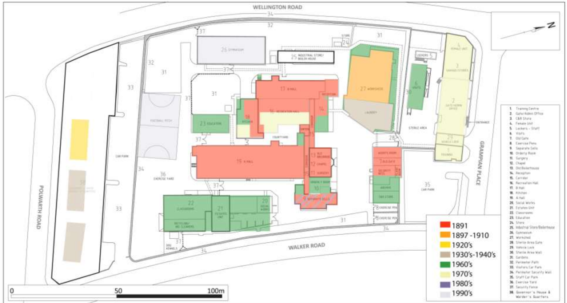
Figure 56: A suggested construction phasing at HMP Aberdeen.
