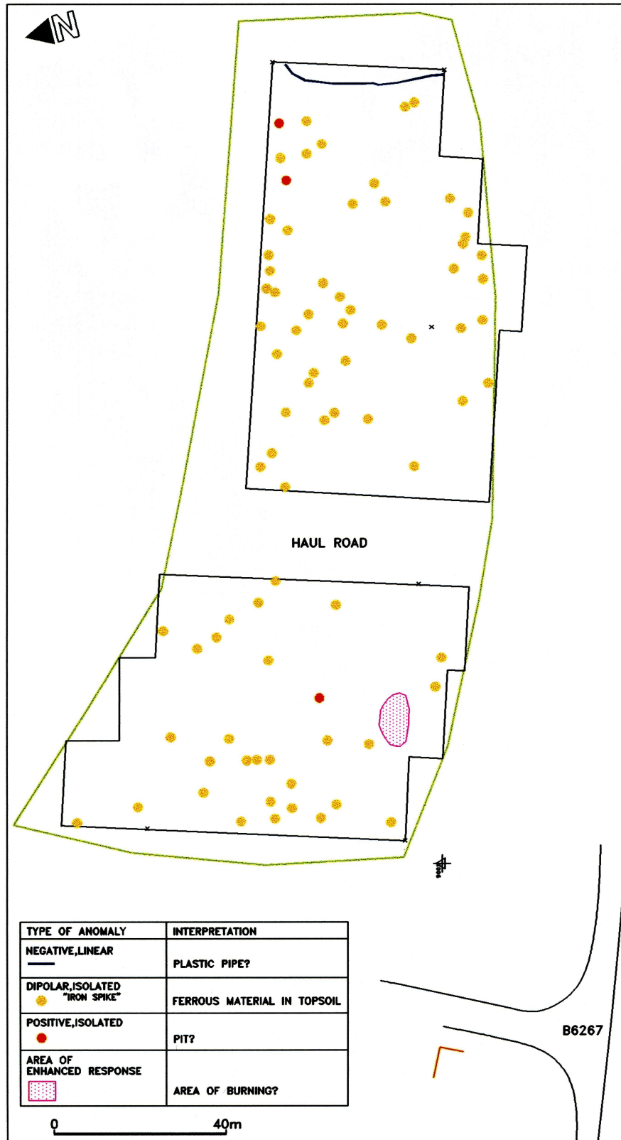
Fig.5 Interpretation of gradiometer data
