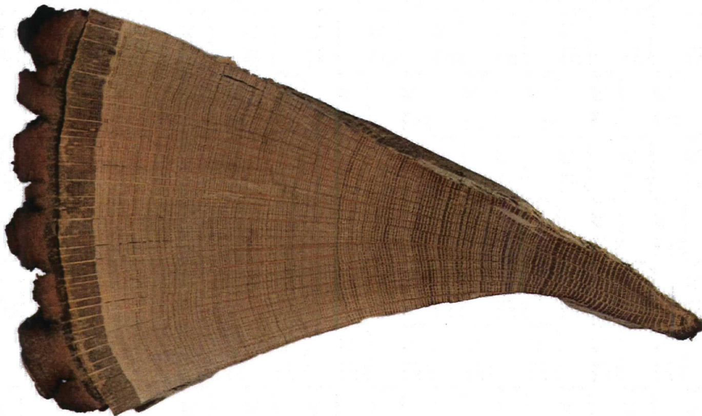
Figure 1: A wedge of oak from a tree felled in 1976. It shows the annual growth rings, one for each year from the innermost ring to the last ring on the outside just inside the bark. The year of each ring can be determined by counting back from the outside ring, which grew in 1976.
