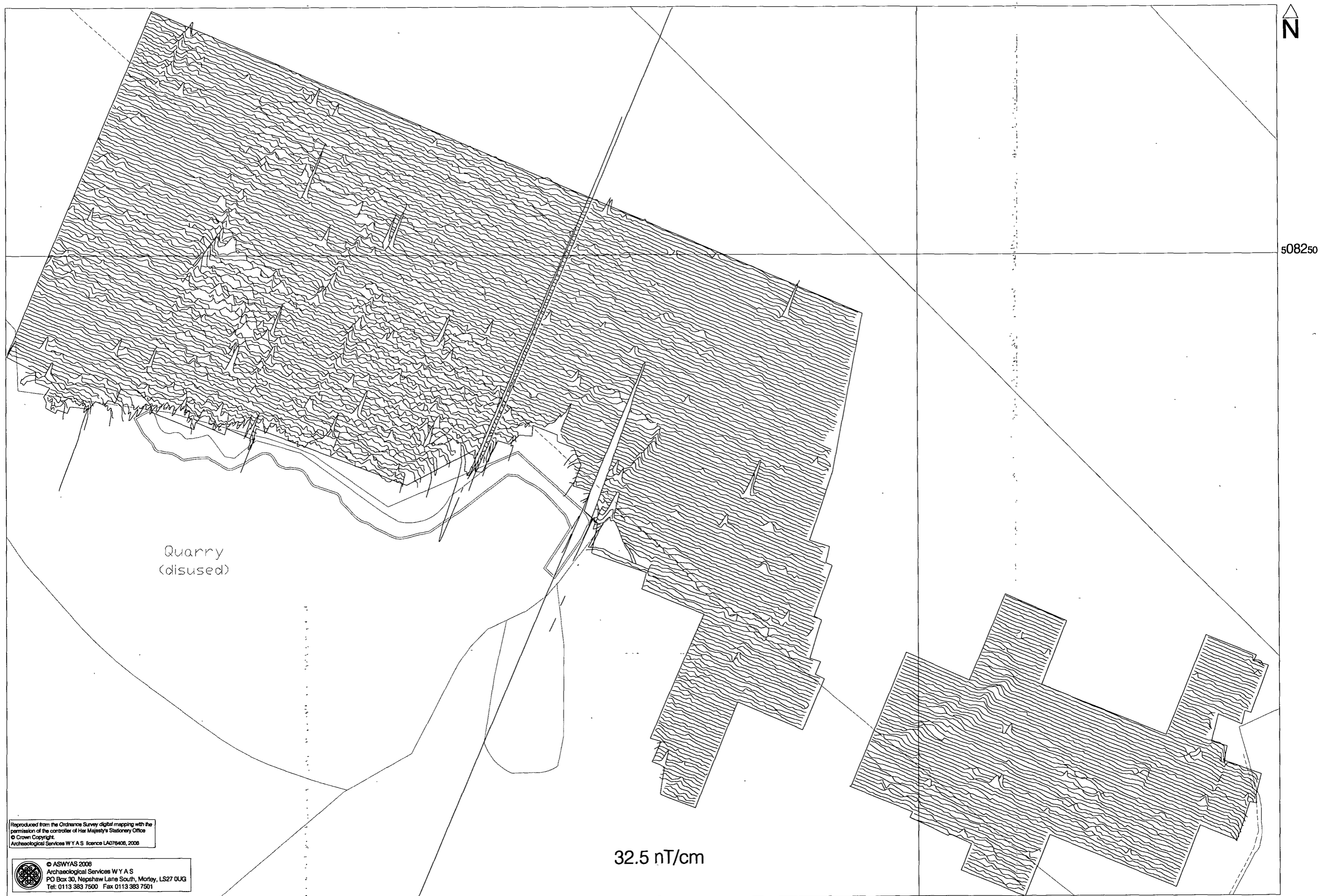
Fig. 4. XY traceplot of unprocessed magnetometer data (1:1000 @ A3)
