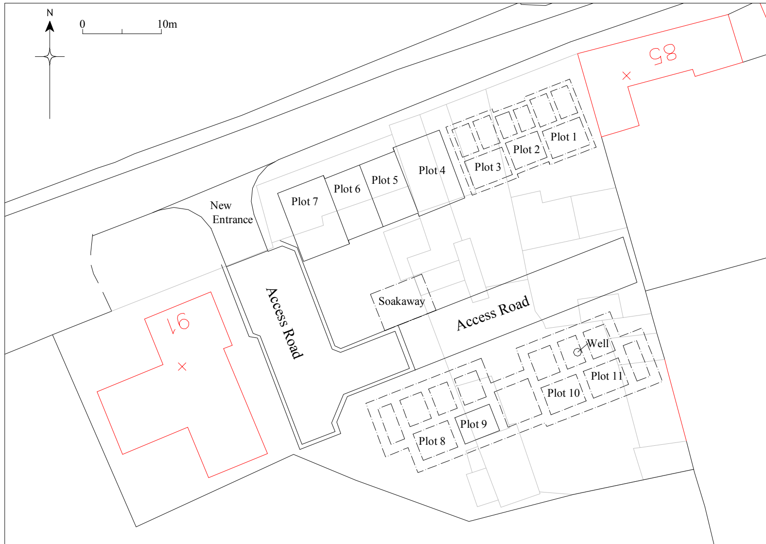
Figure 2 Site plan showing the location of the well, soakaway and foundation trenches within the development with the original site layout in grey.
