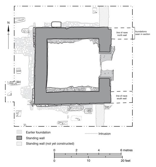
Fig. 12: Construction of the standing tower and associated features
