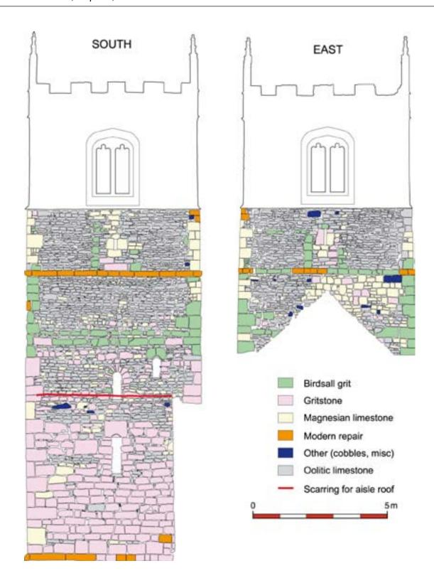
Fig. 13b: South and East elevations showing stone types
