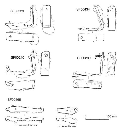
Fig. 8: Iron corner brackets and hinge straps (drawn from x-rays).
