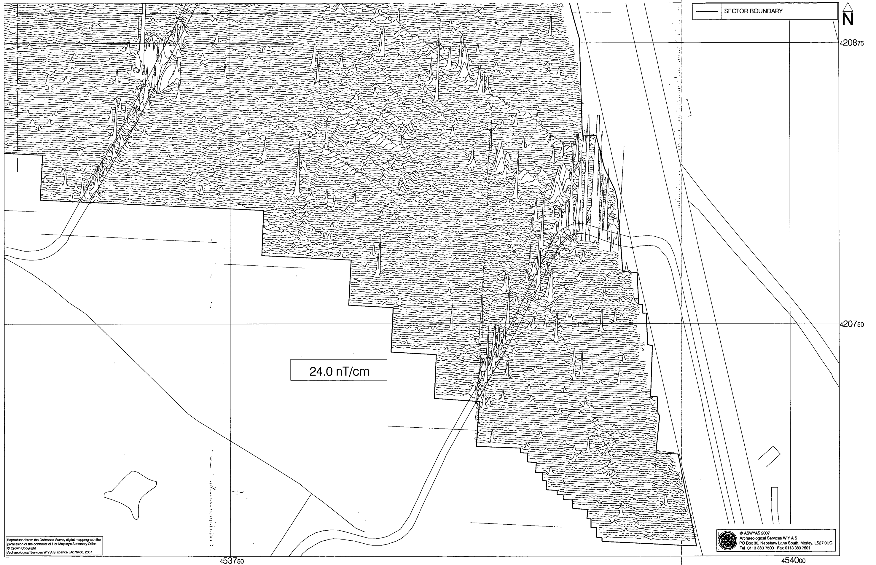
Fig. 10. XY trace plot of unprocessed magnetometer data; south-east sector (1:1000 @ A3)
